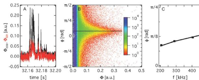
**Fig. 4** (A) The time trace of  $\Phi_{\text{cos}}$  (black) and  $\Phi_{\text{sin}}$  (red) is shown for a representative burst event. (B) Occurrence of the simultaneous measurement of phase delay and amplitude at  $f = 206$  kHz. The average phase delay as extracted from the 2D histogram is plotted in (C). Experimentally measured (squares) and numerically calculated phase delays (solid line).
