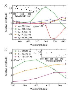
Fig. 9 Decay associated spectra of **C**<sub>4</sub>-**dHONI** ( $c=40~\mu\text{M}$ ) in PhCN in the presence of (a) 200 mM of **NMI** ( $\lambda_{\text{exc}}=360~\text{nm}$ ) and (b) 250  $\mu\text{M}$  of **DBU** ( $\lambda_{\text{exc}}=460~\text{nm}$ ). The insets show the individual  $\chi^2$ -values at each wavelength. The time constants in (b) are given the same labels as the corresponding ones in (a).
