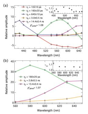
**Fig. 8** Decay associated spectra of **C**<sub>4</sub>**-dHONI** ( $c = 40 \mu M$ ) in MeCN in the presence of (a) 200 mM of **NMI** ( $\lambda_{\rm exc} = 360$  nm) and (b) 250  $\mu M$  of **DBU** ( $\lambda_{\rm exc} = 460$  nm). The insets show the individual  $\chi^2$ -values at each wavelength. The time constants in (b) are given the same labels as the corresponding ones in (a).
