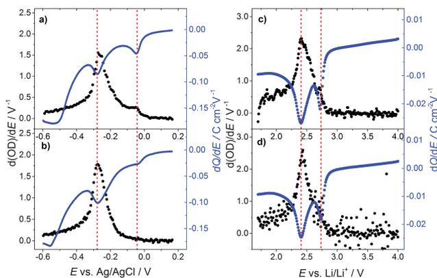
Fig. 3 Differential change of the optical density  $d(\text{OD})/dE$  vs.  $E$  and  $dQ/dE$  (cell current) vs.  $E$  of a WO<sub>3</sub> film for the potential decreasing part of a cyclic voltammogram with a scan rate of  $1 \text{ mV s}^{-1}$  (a) in 0.1 M H<sub>2</sub>SO<sub>4</sub> in H<sub>2</sub>O for the first cycle and (b) the 10th cycle; (c) in 0.2 M LiClO<sub>4</sub> in PC for the first cycle and (d) the 10th cycle.
