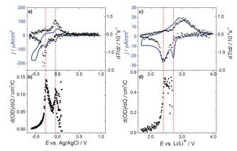
Fig. 2 Transmission change  ${\rm d}T/{\rm d}t$  vs. E and the cyclic voltammogram of a WO $_3$  film in: (a) 0.1 M H $_2$ SO $_4$  in H $_2$ O and (c) 0.2 M LiClO $_4$  in propylene carbonate. Change in the optical density with respect of the amount of (b) inserted protons/electric charge d(OD)/dQ vs. E and (d) inserted lithium ions/electric charge d(OD)/dQ vs. E.
