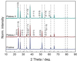
Fig. 6 Diffraction diagrams of the pristine  $WO_3$  film (bottom trace) and the lithium-inserted films formed by galvanostatic discharge down to plateau I at 2.73 V (center trace) and plateau II at 2.45 V (top trace). FTO substrate reflections are marked by gray dashed lines. Indices for reflections attributable to the tetragonal (pristine, plateau I) and cubic phases (plateau II) are depicted.
