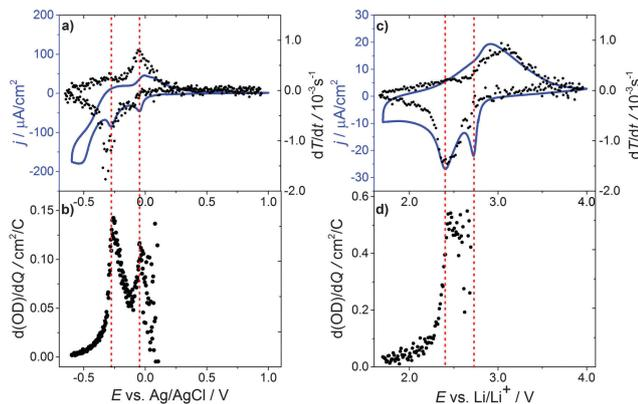
Fig. 2 Transmission change  $dT/dt$  vs.  $E$  and the cyclic voltammogram of a WO<sub>3</sub> film in: (a) 0.1 M H<sub>2</sub>SO<sub>4</sub> in H<sub>2</sub>O and (c) 0.2 M LiClO<sub>4</sub> in propylene carbonate. Change in the optical density with respect of the amount of (b) inserted protons/electric charge  $d(\text{OD})/dQ$  vs.  $E$  and (d) inserted lithium ions/electric charge  $d(\text{OD})/dQ$  vs.  $E$ .
