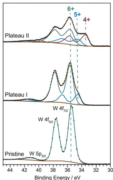
Fig. 5 W 4f core level XP spectra of the pristine  $\text{WO}_3$  film. Lithium inserted  $\text{WO}_3$  films formed by galvanostatic discharge in 0.2 M  $\text{LiClO}_4$  in PC with a constant current of  $-300$  nA down to the first plateau at 2.73 V and the second plateau at 2.45 V.
