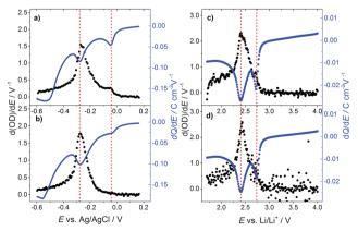
Fig. 3 Differential change of the optical density d(OD)/dE vs. E and dQ/dE (cell current) vs. E of a  $WO_3$  film for the potential decreasing part of a cyclic voltammogram with a scan rate of 1 mV s<sup>-1</sup> (a) in 0.1 M H<sub>2</sub>SO<sub>4</sub> in H<sub>2</sub>O for the first cycle and (b) the 10th cycle; (c) in 0.2 M LiClO<sub>4</sub> in PC for the first cycle and (d) the 10th cycle.
