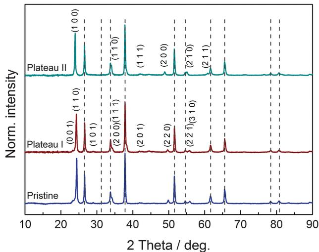
Fig. 6 Diffraction diagrams of the pristine WO<sub>3</sub> film (bottom trace) and the lithium-inserted films formed by galvanostatic discharge down to plateau I at 2.73 V (center trace) and plateau II at 2.45 V (top trace). FTO substrate reflections are marked by gray dashed lines. Indices for reflections attributable to the tetragonal (pristine, plateau I) and cubic phases (plateau II) are depicted.
