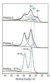
Fig. 5 W 4f core level XP spectra of the pristine  $WO_3$  film. Lithium inserted  $WO_3$  films formed by galvanostatic discharge in 0.2 M LiClO<sub>4</sub> in PC with a constant current of -300 nA down to the first plateau at 2.73 V and the second plateau at 2.45 V.
