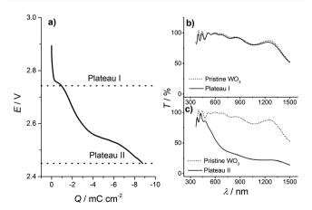
Fig. 4 (a) Correlation of charge and potential for a galvanostatic insertion process of lithium ions into a WO<sub>3</sub> thin film in 0.2 M LiClO<sub>4</sub> in PC for a constant current of −300 nA. Ex situ UV-Vis spectra of WO<sub>3</sub> films inserted up to (b) plateau I at 2.73 V and (c) plateau II at 2.45 V.
