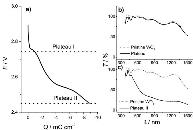
Fig. 4 (a) Correlation of charge and potential for a galvanostatic insertion process of lithium ions into a  $\text{WO}_3$  thin film in 0.2 M  $\text{LiClO}_4$  in PC for a constant current of  $-300$  nA. *Ex situ* UV-Vis spectra of  $\text{WO}_3$  films inserted up to (b) plateau I at 2.73 V and (c) plateau II at 2.45 V.
