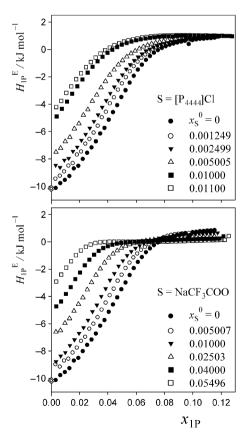
**Fig. 3** Excess partial molar enthalpy,  $H_{1P}^{\rm E}$ , of 1P in 1P–S–H<sub>2</sub>O at 25 °C and given initial salt concentration,  $x_{2}^{\rm G}$ . Diamonds represent  $H_{1P}^{\rm E}$  in dilute solution, as reported by Wadso *et al.*<sup>35</sup>
