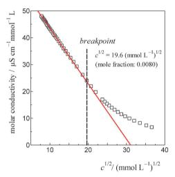
Fig. 9 The isotherm of electric conductivity for aqueous solutions of [P<sub>4444</sub>]CF<sub>3</sub>COO based on the Kohlrausch empirical relation.<sup>42</sup> The break point was estimated to be  $c^{1/2}$  = 19.6 (mmol L<sup>-1</sup>)<sup>1/2</sup> for [P<sub>4444</sub>]CF<sub>3</sub>COO, corresponding to a 0.0080 mole fraction of the IL.
