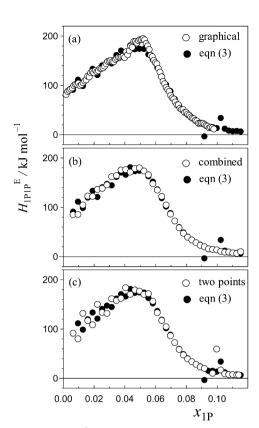
**Fig. 4** Comparison of  $H_{1P1P}^{E}$  pattern for the binary (1-propanol- $H_{2}O$ ) mixture calculated based on differentiation using eqn (3) (solid circles) with those using other evaluation methods (open circles); (a) typical graphical evaluation normally exercised for 1P-probing studies,<sup>34</sup> (b) combination of calculation using eqn (3) and graphical evaluation, (c) simple derivative using two data points with  $\delta x_{1P} \approx 0.006$ .
