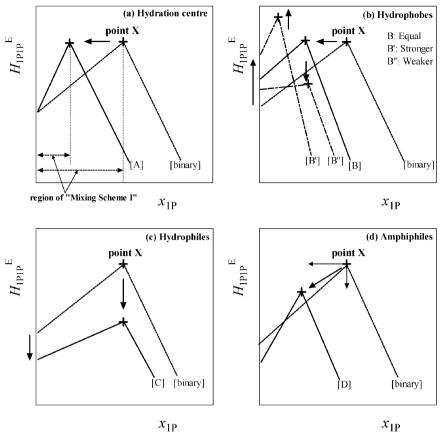
Fig. 2 Induced changes of  $H_{1P1P}^{E}$  pattern in the presence of various types of solute S. [binary] represents the binary  $1P-H_2O$  system without test solute S. (a) Effects of the hydration centre on the pattern per unit increase in test sample S. Region of Mixing Scheme I is defined as  $x_{1P} = 0$  to  $x_{1P}$  at point X, as described on the horizontal axis, (b) the effects of hydrophobes, (c) hydrophiles and (d) amphiphiles
