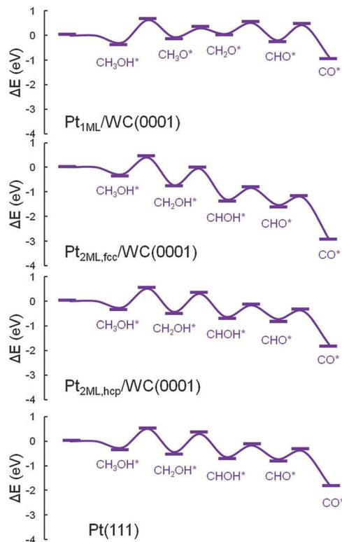
**Fig. 3** Energy profiles for the dehydrogenation of methanol from CH<sub>3</sub>OH\* to CO\* + 4H\* over Pt<sub>1ML</sub>/WC(0001), Pt<sub>2ML,fcc</sub>/WC(0001), Pt<sub>2ML,hcp</sub>/WC(0001) and Pt(111) surfaces.
