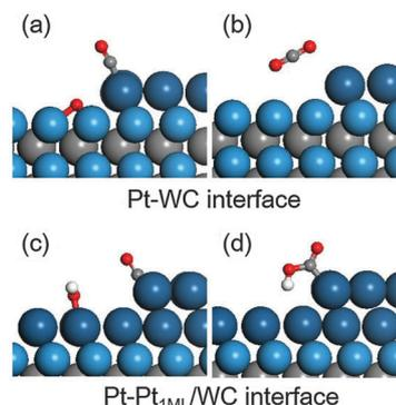
**Fig. 5** Optimized structures for surface CO\* oxidation at the Pt–WC(0001) and Pt–Pt<sub>1ML</sub>/WC(0001) interfaces: (a) CO\*/Pt and O\*/WC; (b) CO<sub>2</sub> product; (c) CO\*/Pt-edge and OH\*/Pt<sub>1ML</sub>/WC; (d) COOH\*/Pt-edge.
