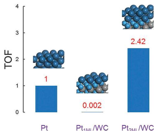
Fig. 6 The calculated normalized turnover frequency TOF in the electro-oxidation of methanol on Pt(111),  $\text{Pt}_{1\text{ML}}/\text{WC}(0001)$  and  $\text{Pt}_{2\text{ML}}/\text{WC}(0001)$  surfaces, respectively.
