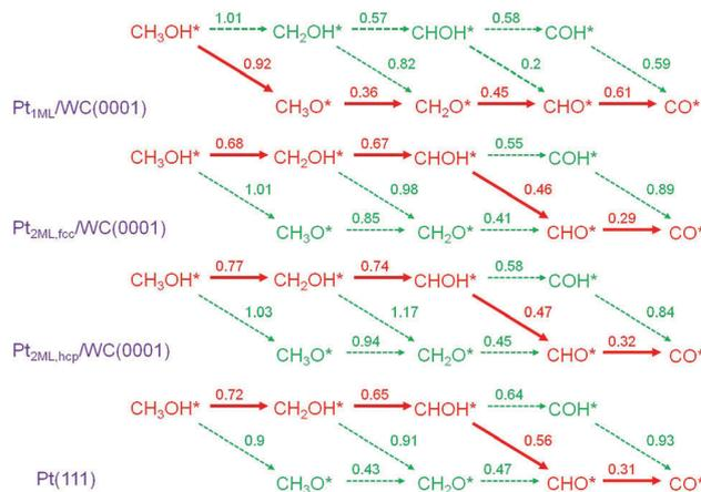
Fig. 2 Reaction networks and the calculated reaction barriers (in eV) for methanol dehydrogenation from CH<sub>3</sub>OH\* to CO\* + 4H\* over Pt<sub>1ML</sub>/WC(0001), Pt<sub>2ML,fcc</sub>/WC(0001), Pt<sub>2ML,hcp</sub>/WC(0001) and Pt(111) surfaces. The paths in red color present the favored pathways in methanol dehydrogenation with the intermediates involved and the barriers shown.
