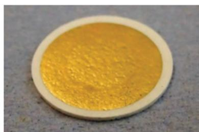
Fig. 1 Pressed MOF pellet with 80 nm gold layer.
