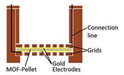
Fig. 2 Cross section schema of the sample holder.
