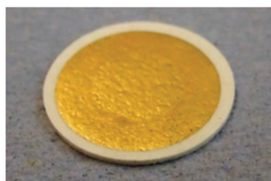
Fig. 1 Pressed MOF pellet with 80 nm gold layer.
