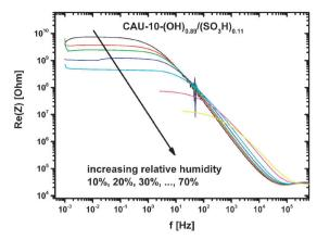
Fig. 4 Re(Z) of CAU-10-O/S at different relative humidity
