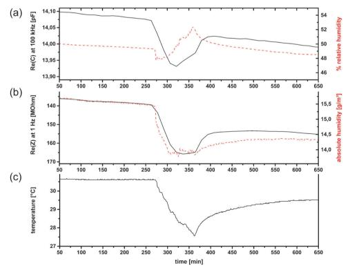
Fig. 11 Application test no. 2 of CAU-10-N/S during the opening of a window from minute 270 to 300. Re(C) at 100 kHz compared to relative humidity (a); Re(Z) at 1 Hz (reversed scale) compared to absolute humidity (b); and temperature (c); (humidity in dashed lines).
