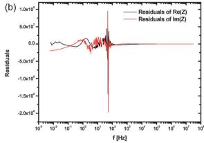
(a) Measured data for CAU-10-O/S at 30% r.h. (dots), fitted with Cole-Cole model (black, dashed line) and fitted with Havriliak-Negami model (red line). Please note the different axis scaling. (b) Residual plot for the exemplarily given fit in (a). The highest peaks are due to 50 Hz noise.
