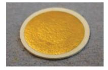
Fig. 1 Pressed MOF pellet with 80 nm gold layer.
