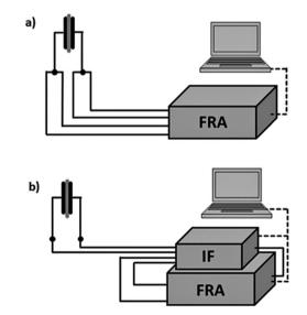
Fig. 3 Set-up (a) in 4-point-arrangement with only the FRA and (b) enhanced with dielectric interface for highly ohmic sample conditions.
