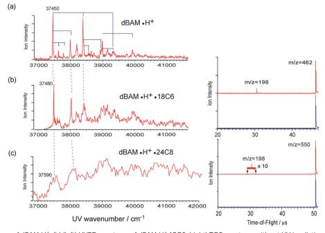
Fig. 5 (a) UVPD spectrum of dBAM·H $^+$ . (b) (left) UVPD spectrum of dBAM·H $^+$ ·18C6. (right) TOF spectrum without UV irradiation (blue) and with UV fixed at 37 481 cm $^{-1}$  (red). The ion intensity is normalized relative to parent ion intensity. (c) (left) UVPD spectrum of dBAM·H $^+$ ·24C8. (right) TOF spectrum without UV irradiation (blue) and with UV fixed at 37 594 cm $^{-1}$  (red). The ion intensity is normalized relative to parent ion intensity.
