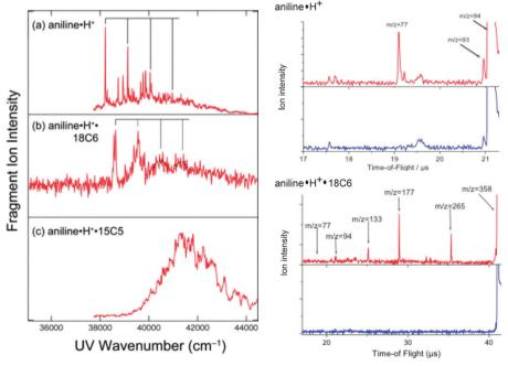
Fig. 1 (left) UVPD spectra of (a) aniline·H+, (b) aniline·H+.18C6, and (c) aniline·H+.15C5. (right) TOF spectra of aniline·H+ and aniline·H+.18C6, without UV irradiation (blue) and with UV irradiation fixed at the band origins (red). The solid black lines in (a) and (b) show the progression with an interval of  $\sim$  920 cm<sup>-1</sup> assigned to the ring breathing mode
