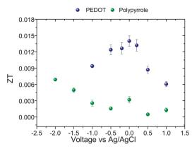
Fig. 5 ZT of PEDOT and PPy as a function of applied potential at 300 K.
