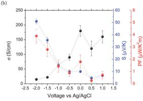
Fig. 4 Electrical conductivity, Seebeck coefficient and power factor of (a) PEDOT and (b) PPy as a function of voltage referred to the Ag/AgCl electrode
