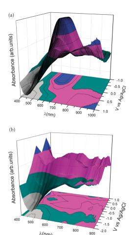
Fig. 3 UV-Vis spectra of: (a) PEDOT and (b) polypyrrole as a function of different applied voltages vs. Ag/AgCl on ITO coated glass electrodeposited polymer films.
