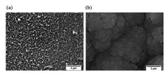
Fig. 1 SEM images of: (a) PEDOT and (b) PPy film surfaces after electrochemical polymerization.
