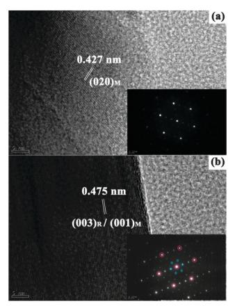
Fig. 2 HRTEM images of (a) Li<sub>1.2</sub>Mn<sub>0.54</sub>Ni<sub>0.13</sub>Co<sub>0.13</sub>O<sub>2</sub> and (b) Li<sub>1.2</sub>Mn<sub>0.39</sub>-Ti<sub>0.15</sub>Ni<sub>0.13</sub>Co<sub>0.13</sub>O<sub>2</sub>. Insets show SAED patterns of the corresponding materials
