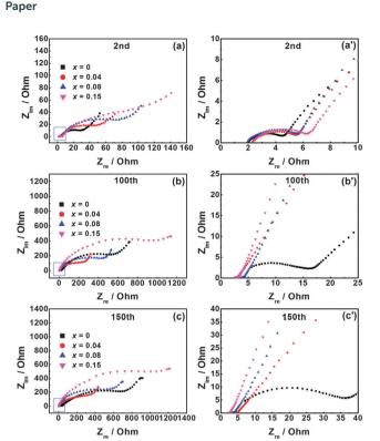
Fig. 12 Nyquist plots of Li/Li $_{1.2}$ Mn $_{0.54-x}$ Ti $_x$ Ni $_{0.13}$ Co $_{0.13}$ O $_2$  (x=0,0.04,0.08, and 0.15) during cycling at a current density of 200 mA g $^{-1}$ . The frequency ranges were 100 000-0.01 Hz for the 2nd cycle, and 100 000-0.001 Hz for the 100th and 150th cycles.
