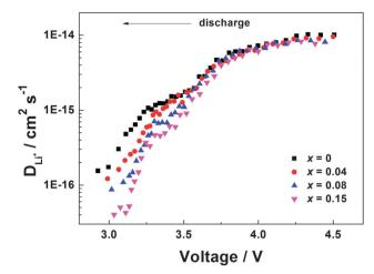
**Fig. 13** Diffusion coefficients of Li<sup>+</sup> for Li<sub>1.2</sub>Mn<sub>0.54-x</sub>Ti<sub>x</sub>Ni<sub>0.13</sub>Co<sub>0.13</sub>O<sub>2</sub> (x = 0, 0.04, 0.08, and 0.15) during the 3rd discharge process.
