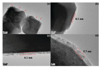
Fig. 11 TEM images of  $Li_{1.2}Mn_{0.54-x}Ti_xNi_{0.13}Co_{0.13}O_2$  materials after 150 cycles at a current density of 200 mA  $g^{-1}$ . (a) x = 0, (b) x = 0.04, (c) x = 0.040.08, and (d) x = 0.15.
