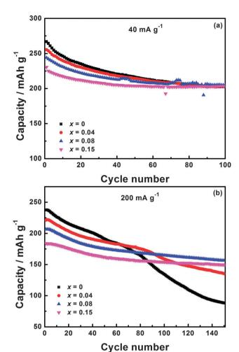
Fig. 4 Cycling performance of  $\rm Li_{1.2}Mn_{0.54-x}Ti_xNi_{0.13}Co_{0.13}O_2$  (x=0,0.04,0.08, and 0.15) at current densities of (a) 40 mA  $\rm g^{-1}$  and (b) 200 mA  $\rm g^{-1}$  over 2–4.7 V.
