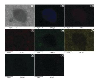
Fig. 10 (a) SEM image of the "dark" surface compounds on a cycled Li<sub>1,2</sub>Mn<sub>0,54</sub>Ni<sub>0,13</sub>Co<sub>0,13</sub>O<sub>2</sub> electrode and the corresponding EDS mappings of (b) F, (c) P, (d) O, (e) C, (f) Mn, (g) Co, and (h) Ni.
