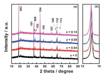
Fig. 1 XRD patterns of  $Li_{1.2}Mn_{0.54-x}Ti_xNi_{0.13}Co_{0.13}O_2$  (x = 0, 0.04, 0.08,
