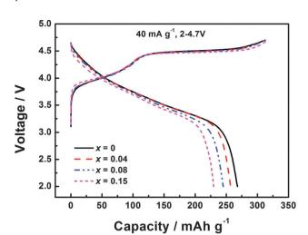
Fig. 3 Initial charge–discharge profiles of  $Li_{1.2}Mn_{0.54-x}Ti_xNi_{0.13}Co_{0.13}O_2$  (x = 0, 0.04, 0.08, and 0.15) at the current density of 40 mA  $g^{-1}$  over 2–4.7 V.
