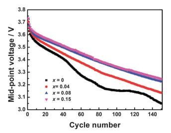
**Fig. 6** Mid-point voltage of  $Li_{1.2}Mn_{0.54-x}Ti_xNi_{0.13}Co_{0.13}O_2$  (x=0, 0.04, 0.08, and 0.15) materials cycled at a current density of 200 mA  $g^{-1}$ .
