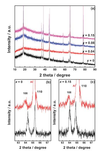
Fig. 8 XRD patterns of (a)  $Li_{1.2}Mn_{0.54-x}Ti_xNi_{0.13}Co_{0.13}O_2$  (x = 0, 0.04, 0.08,and 0.15) electrodes after 150 cycles at a current density of 200 mA g (b) and (c) A comparison of XRD patterns between the pristine material (black line) and the cycled electrode (red line) for Li<sub>1.2</sub>Mn<sub>0.54</sub>Ni<sub>0.13</sub>Co<sub>0.13</sub>O<sub>2</sub> and  $Li_{1.2}Mn_{0.39}$   $Ti_{0.15}Ni_{0.13}Co_{0.13}O_2$ , respectively.
