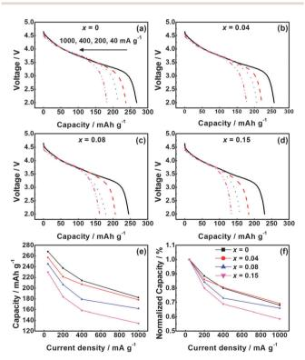
Fig. 7 Rate capabilities of  $Li_{1.2}Mn_{0.54-x}Ti_xNi_{0.13}Co_{0.13}O_2$  with the Ti content of (a) x = 0, (b) x = 0.04, (c) x = 0.08, and (d) x = 0.15. A comparison of discharge capacity and normalized discharge capacity for different materials is shown in (e) and (f), respectively
