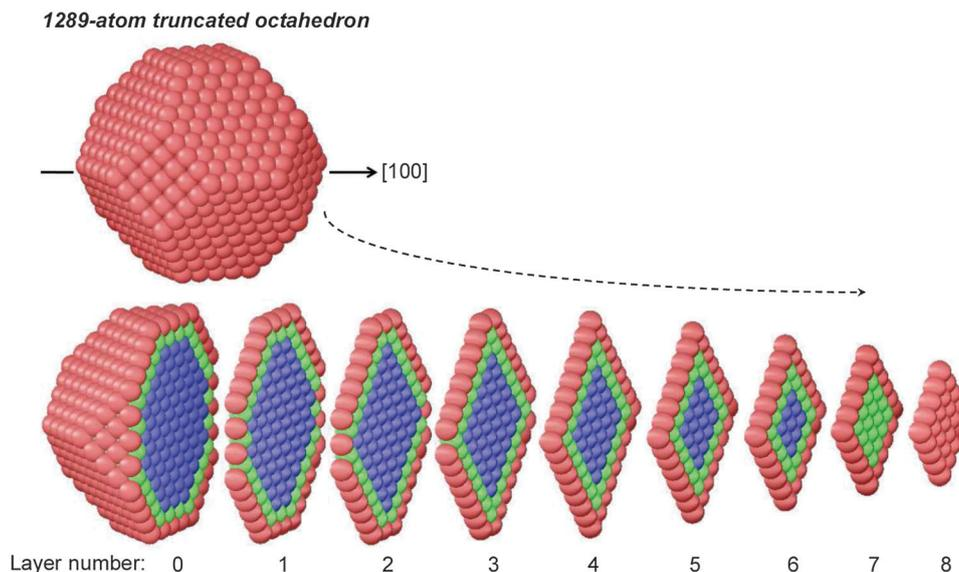
**Fig. 1** Illustration of the coarse-grained layer model (CGLM): the number of concentration variables is reduced by grouping together atomic sites within layers perpendicular to a chosen axis. Distinct concentration variables correspond to: (a) surface sites (red) having four different coordinations (vertices, edges, (100) and (111) faces), (b) core sites in two locations: the inner-core (blue) and the subsurface (green).
