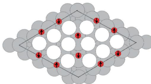
Fig. 9 The atomic structure of the  $p(4 \times 4)$  reconstruction. The silver atoms in the  $Ag_6$  units are shaded white. Oxygen atoms are shown as small red circles. The arrows show which oxygen atoms lie above the  $Ag_6$  plane (up arrows) and below the  $Ag_6$  plane (down arrows). Subsurface silver atoms are shown by way of large grey circles.
