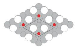
**Fig. 20** Substitutional oxygen with  $(\sqrt{3} \times \sqrt{3})$  periodicity. The silver surface atoms are shaded white to distinguish them from the underlying (grey) silver atoms. The oxygen atoms, shown as small red circles, are displaced from the substitutional sites.
