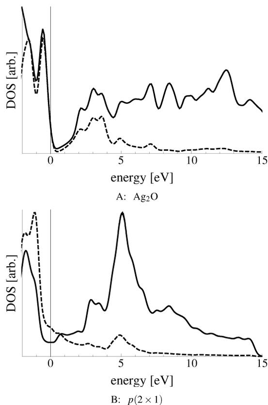
Fig. 28 (A) Density of O p states (dashed line) and the total density of states on Ag (solid line) in  $\text{Ag}_2\text{O}$ . (B) Density of O p (dashed line) and all Ag (solid line) states in the  $p(2 \times 1)$  reconstruction of the Ag(110) surface. In both cases the Fermi energy has been set to zero and is shown using a vertical line.
