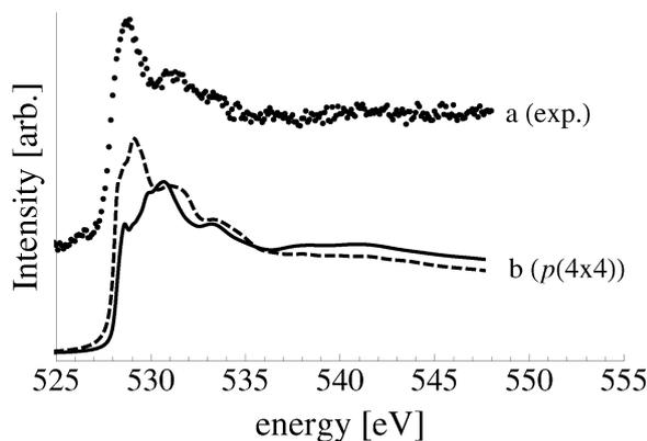
Fig. 30 The O K-edge spectra of the  $p(4 \times 4)$  reconstruction of the Ag(111) surface calculated with (solid line) and without (dashed line) a core hole on the absorbing atom (b). The experimental results are shown for comparison (a).
