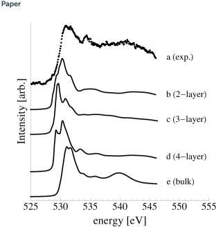
Fig. 19 Measured O K-edge spectrum of  $Ag_2O$  (a). The calculated O K-edge spectra of two (b), three (c), and four (d) layer oxide-like structures on the Ag(111) surface.
