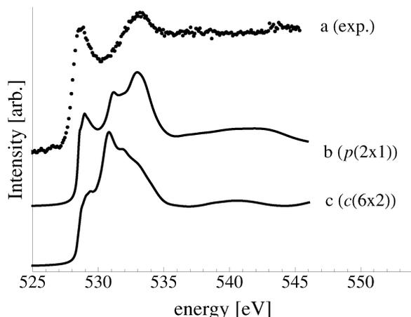
Fig. 5 Waterfall plot of the measured O K-edge spectrum of the Ag(110) surface exposed to  $10^{-4}$  mbar O<sub>2</sub> pressure for 22 minutes at 423 K (a). Calculated O K-edge spectra of the  $p(2 \times 1)$  added row (b) and of the  $c(6 \times 2)$  added strand reconstructions (c) on the Ag(110) surface.
