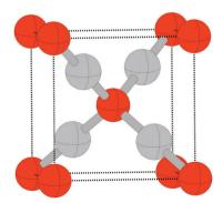
Fig. 25 The atomic structure of Ag<sub>2</sub>O. The oxygen atoms (red) form a bcc lattice and the silver atoms (light grey) form an interpenetrating fcc lattice.
