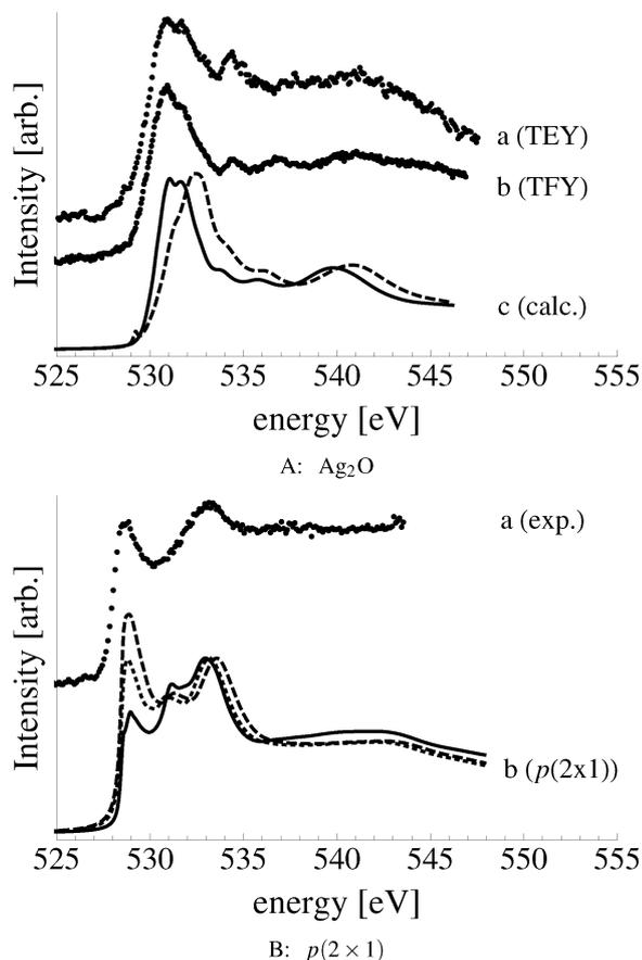
Fig. 29 O K-edge spectra of Ag<sub>2</sub>O (A) and oxygen in the  $p(2 \times 1)$  reconstruction of the Ag(110) (B) calculated with (solid line) and without (dashed line) a core hole on the absorbing atom. The dotted line in (B) was generated by changing how the occupied states are removed from the spectrum in the absence of a core hole. The experimental results are shown for comparison.
