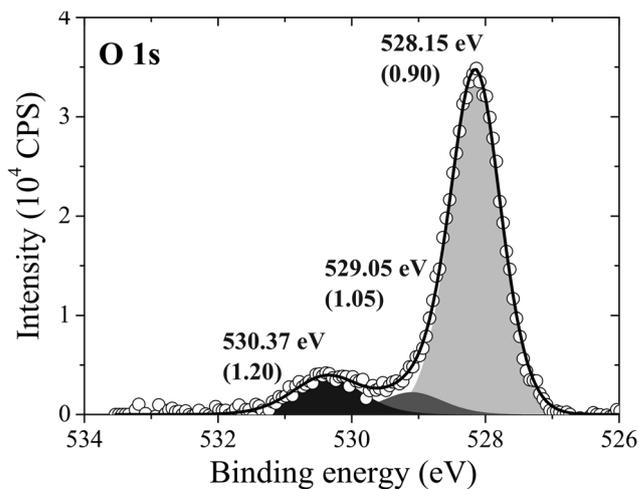
Fig. 14 The measured O<sub>1s</sub> spectrum of Ag(111) after dosing oxygen for 48 minutes at 423 K and  $10^{-4}$  mbar O<sub>2</sub> pressure.
