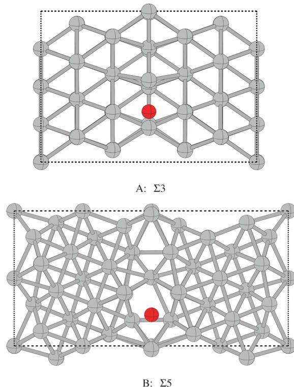
Fig. 23 Atomic structure of the  $\Sigma 3$  (A) and  $\Sigma 5$  (B) grain boundaries in silver viewed down the boundary. In both images, the grain boundary is in the center of the simulation cell. The silver atoms are shaded light grey and nearest neighboring bonds are shown. The adsorbed oxygen is shaded red. The dotted lines represent the edges of the simulation cell.
