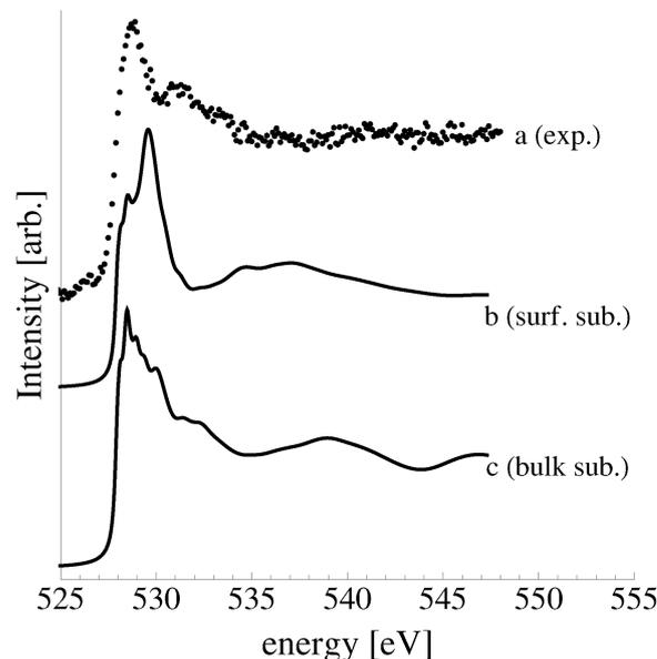
Fig. 21 The measured spectrum for Ag(111) exposed to  $O_2$  (a). The O K-edge spectrum of surface substitutional oxygen with  $(\sqrt{3} \times \sqrt{3})$  periodicity (b) and of bulk substitutional oxygen (c).
