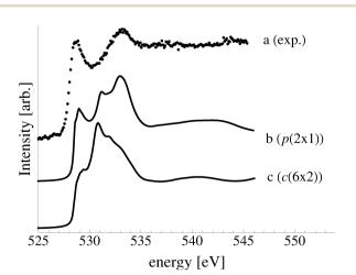
Fig. 5 Waterfall plot of the measured O K-edge spectrum of the Ag(110) surface exposed to  $10^{-4}$  mbar  $O_2$  pressure for 22 minutes at 423 K (a). Calculated O K-edge spectra of the  $p(2\times1)$  added row (b) and of the  $c(6\times2)$  added strand reconstructions (c) on the Ag(110) surface.
