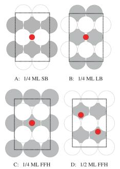
Fig. 3 Atomic structure of 1/4 ML oxygen on the short bridge (SB) (A), long bridge (LB) (B), and four-fold hollow (FFH) sites (C), along with 1/2 ML oxygen on the four-fold hollow sites (D). The coloring is the same as Fig. 1.
