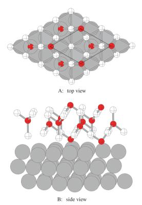
Fig. 18 Atomic positions in the low energy oxide-like structures on the Ag(111) surface viewed in the direction normal to the surface (A) and as a slice through the surface (B). The surface silver atoms are shaded white and the unit cell is indicated by way of the black dashed line. For clarity, thick lines are used to indicate bonds between nearest neighbors silver and oxygen atoms in the oxide-like layer.
