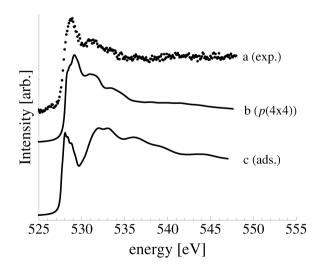
Fig. 15 The O K-edge spectrum measured after dosing the Ag(111) single crystal with oxygen for 48 minutes at 423 K and  $10^{-4}$  mbar  $O_2$  pressure (a). The calculated spectra of oxygen in the  $p(4 \times 4)$  reconstruction on the Ag(111) surface (b) and 1/16 ML unreconstructed chemisorbed atomic oxygen (c).
