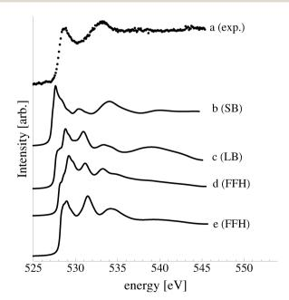
**Fig. 6** The measured O K-edge spectrum of the Ag(110) surface exposed to  $10^{-4}$  mbar  $\rm O_2$  pressure for 22 minutes at 423 K (a). The calculated O K-edge spectra of 1/4 ML oxygen on the SB (b), LB (c), and FFH (d) sites of the Ag(110) surface, along with 1/2 ML oxygen on the FFH sites (e).
