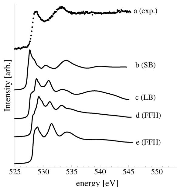
Fig. 6 The measured O K-edge spectrum of the Ag(110) surface exposed to  $10^{-4}$  mbar O<sub>2</sub> pressure for 22 minutes at 423 K (a). The calculated O K-edge spectra of 1/4 ML oxygen on the SB (b), LB (c), and FFH (d) sites of the Ag(110) surface, along with 1/2 ML oxygen on the FFH sites (e).
