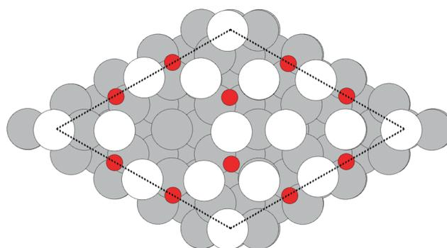
Fig. 24 The atomic structure of the  $p(4 \times 4)$  reconstruction suggested by Carlisle *et al.*<sup>113</sup> The surface silver atoms are shaded white. Oxygen atoms are shown as red and the subsurface silver as grey. The dotted line shows the surface unit cell.
