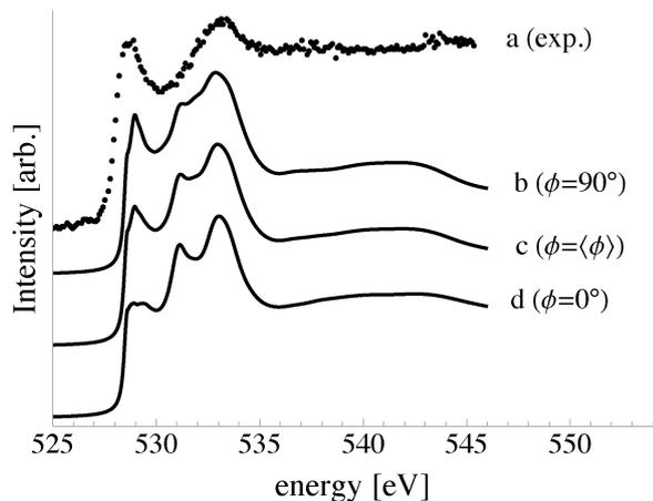
Fig. 27 The measured (a) O K-edge spectrum of oxygen adsorbed on the Ag(110) surface (a) and the computed O K-edge spectra of oxygen in the  $p(2 \times 1)$  reconstruction on the Ag(110) surface (b–d) with varying angle  $\phi$ , the angle between the in-plane component of the  $\mathbf{E}$  vector of the incident radiation and the  $[1\bar{1}0]$  direction along the surface.
