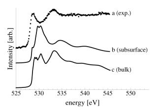
**Fig. 7** The measured O K-edge spectrum of the Ag(110) surface exposed to  $10^{-4}$  mbar  $\rm O_2$  pressure for 22 minutes at 423 K (a). The calculated O K-edge spectra of 1/4 ML oxygen in the octahedral subsurface sites under the Ag(110) surface (b) and in the bulk (c).
