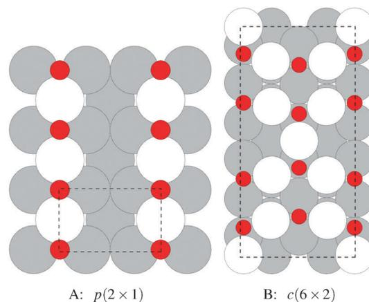
Fig. 1 The atomic structure of the  $p(2 \times 1)$  added row reconstruction (A) and the  $c(6 \times 2)$  added strand (B) on the Ag(110) surface. The silver atoms incorporated into the reconstructions are shaded white and the others grey. Oxygen atoms are shown as small red circles. The unit cells are shown by way of the black dashed lines.
