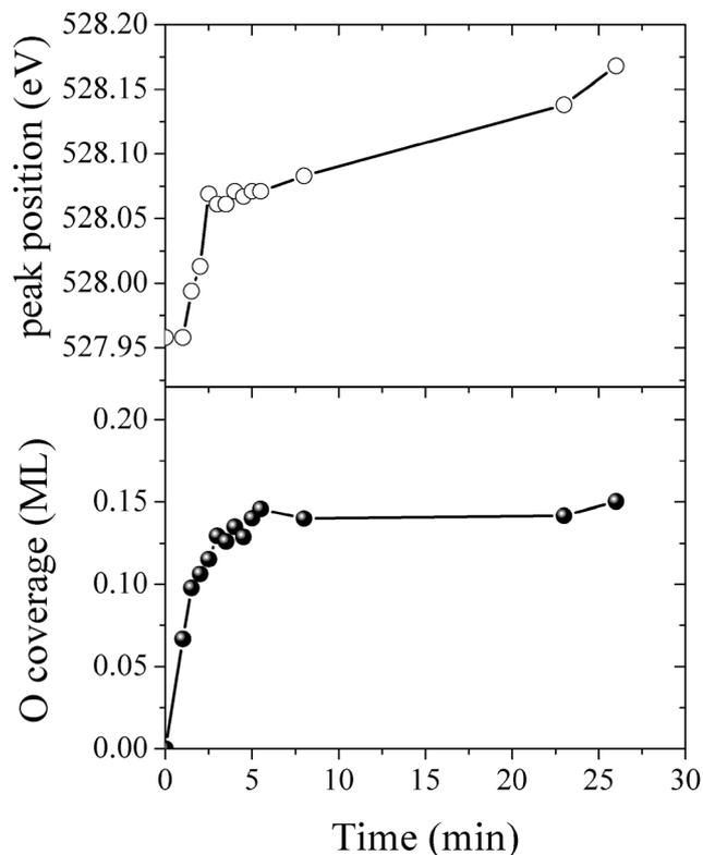
Fig. 13 The O/Ag ratio (top) and the O<sub>1s</sub> peak position (bottom) measured as a function of time for the Ag(111) surface exposed to  $4 \times 10^{-4}$  mbar O<sub>2</sub> pressure at 423 K.
