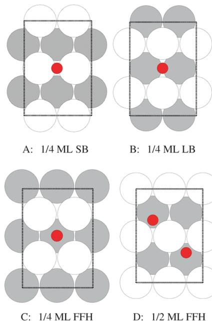
**Fig. 3** Atomic structure of 1/4 ML oxygen on the short bridge (SB) (A), long bridge (LB) (B), and four-fold hollow (FFH) sites (C), along with 1/2 ML oxygen on the four-fold hollow sites (D). The coloring is the same as Fig. 1.
