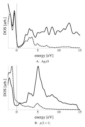
Fig. 28 (A) Density of O p states (dashed line) and the total density of states on Ag (solid line in Ag<sub>2</sub>O). (B) Density of O p (dashed line) and all Ag (solid line) states in the  $p(2\times 1)$  reconstruction of the Ag(110) surface. In both cases the Fermi energy has been set to zero and is shown using a vertical line.
