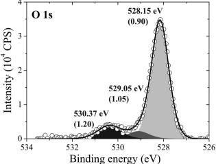
Fig. 14 The measured  $O_{1s}$  spectrum of Ag(111) after dosing oxygen for 48 minutes at 423 K and  $10^{-4}$  mbar  $O_2$  pressure.
