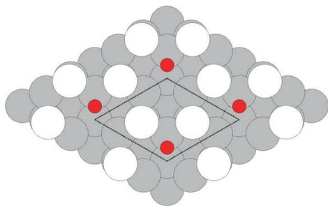
Fig. 20 Substitutional oxygen with  $(\sqrt{3} \times \sqrt{3})$  periodicity. The silver surface atoms are shaded white to distinguish them from the underlying (grey) silver atoms. The oxygen atoms, shown as small red circles, are displaced from the substitutional sites.
