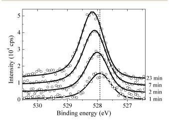
**Fig. 12** The measured  $O_{1s}$  spectrum of the Ag(111) surface exposed to  $4\times 10^{-4}$  mbar  $O_2$  pressure at 423 K for 1, 2, 7 and 23 minutes (from bottom to top). The noise in the measured spectrum is the result of the fast scan rate, 1 scan per minute, required to follow the short time scale evolution of the oxygen species. The vertical dashed line shows the  $O_{1s}$  binding energy obtained for chemisorbed atomic oxygen.
