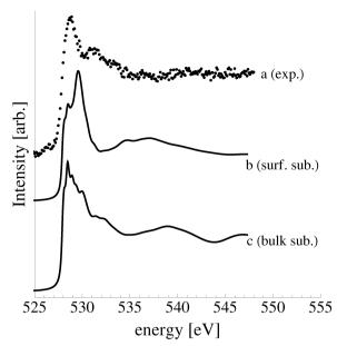
Fig. 21 The measured spectrum for Ag(111) exposed to O<sub>2</sub> (a). The O K-edge spectrum of surface substitutional oxygen with  $\left(\sqrt{3}\times\sqrt{3}\right)$  periodicity (b) and of bulk substitutional oxygen (c).
