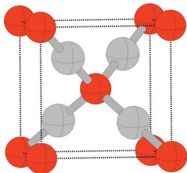
Fig. 25 The atomic structure of  $\text{Ag}_2\text{O}$ . The oxygen atoms (red) form a bcc lattice and the silver atoms (light grey) form an interpenetrating fcc lattice.
