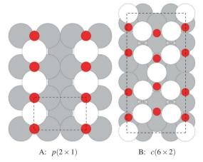
Fig. 1 The atomic structure of the  $p(2 \times 1)$  added row reconstruction (A) and the  $c(6 \times 2)$  added strand (B) on the Aq(110) surface. The silver atoms incorporated into the reconstructions are shaded white and the others grey. Oxygen atoms are shown as small red circles. The unit cells are shown by way of the black dashed lines.
