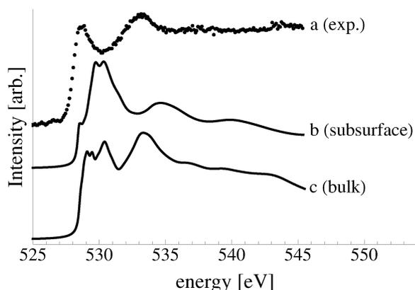
Fig. 7 The measured O K-edge spectrum of the Ag(110) surface exposed to  $10^{-4}$  mbar  $O_2$  pressure for 22 minutes at 423 K (a). The calculated O K-edge spectra of 1/4 ML oxygen in the octahedral subsurface sites under the Ag(110) surface (b) and in the bulk (c).
