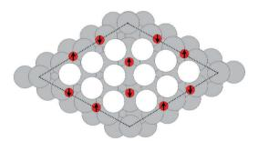
Fig. 9 The atomic structure of the  $p(4 \times 4)$  reconstruction. The silver atoms in the Ag<sub>6</sub> units are shaded white. Oxygen atoms are shown as small red circles. The arrows show which oxygen atoms lie above the Ag<sub>6</sub> plane (up arrows) and below the Ag<sub>6</sub> plane (down arrows). Subsurface silver atoms are shown by way of large grey circles.
