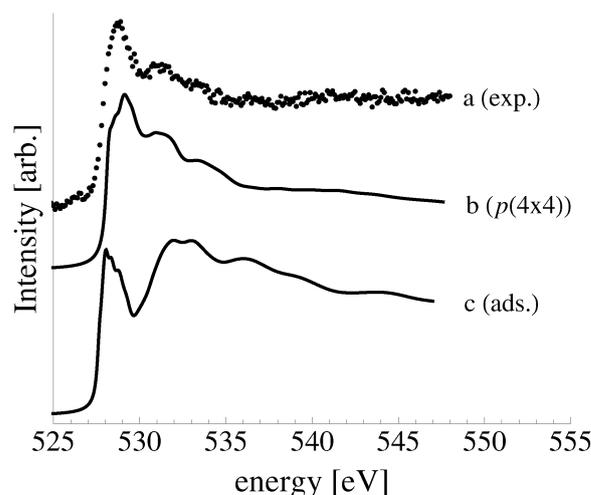
Fig. 15 The O K-edge spectrum measured after dosing the Ag(111) single crystal with oxygen for 48 minutes at 423 K and  $10^{-4}$  mbar O<sub>2</sub> pressure (a). The calculated spectra of oxygen in the  $p(4 \times 4)$  reconstruction on the Ag(111) surface (b) and 1/16 ML unreconstructed chemisorbed atomic oxygen (c).
