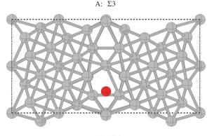
Fig. 23 Atomic structure of the  $\Sigma 3$  (A) and  $\Sigma 5$  (B) grain boundaries in silver viewed down the boundary. In both images, the grain boundary is in the center of the simulation cell. The silver atoms are shaded light grey and nearest neighboring bonds are shown. The adsorbed oxygen is shaded red. The dotted lines represent the edges of the simulation cell.
