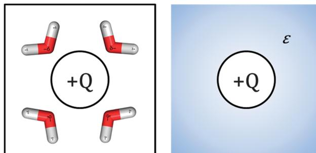
Fig. 3 (left) Water molecules reorient themselves to preferentially point the negative end of their dipole towards the positive solute charge (+ $Q$ ). (right) The system is modelled with a continuous polarisable field. Polarizability is represented by the bulk dielectric constant,  $\epsilon$ .
