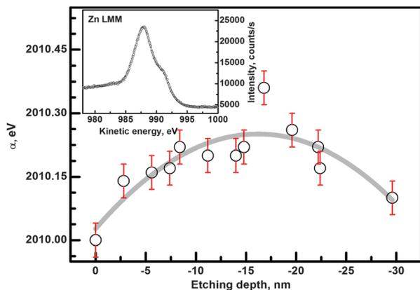
Fig. 5 Determined  $\alpha$ -parameter as a function of ion etching depth for the 4c sample. The depth dependence was fitted with a polynomial to show the trend in the data. The inset shows the Auger Zn LMM energy region.
