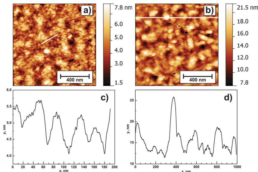
Fig. 1 AFM images of 1  $\mu\text{m}$   $\times$  1  $\mu\text{m}$  height obtained for samples 1c (a) and 4c (b). Panels (c) and (d) show the extracted profiles marked with white lines in the corresponding images.
