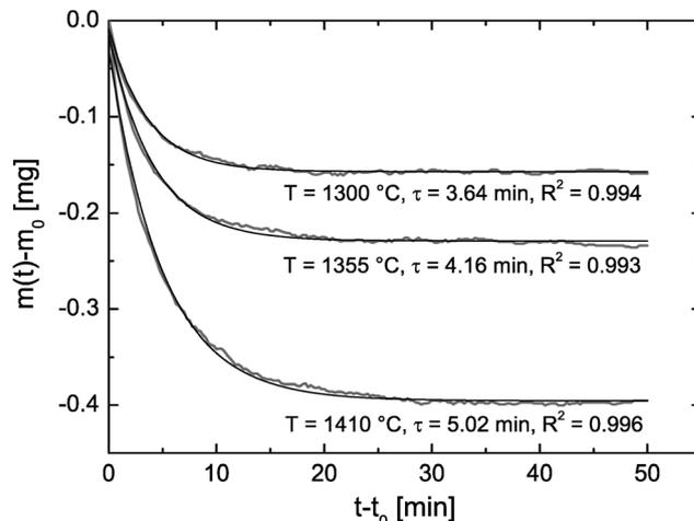
Fig. 8 Isothermal time dependence of the mass loss during the reduction cycles R1–R3 in Fig. 7 where  $m_0$  is the mass at time  $t_0$  when the temperature starts to become constant. Time constants,  $\tau$ , to reach mass equilibrium are evaluated by fit eqn (13) where the  $R^2$  values quantify the fit quality.
