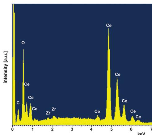
Fig. 6 EDS analysis of the sintered CeO<sub>2</sub> pellet.
