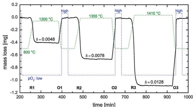
Fig. 7 Reduction cycles (R1–R3) and oxidation cycles (O1–O3) during thermogravimetric analysis of a nominally undoped polycrystalline  $\text{CeO}_2$  pellet (see Table 1). Dashed lines show the time dependence of the temperature and the oxygen partial pressure  $p_{\text{O}_2}$  (low:  $7 \times 10^{-4}$  atm, high: 0.4 atm).
