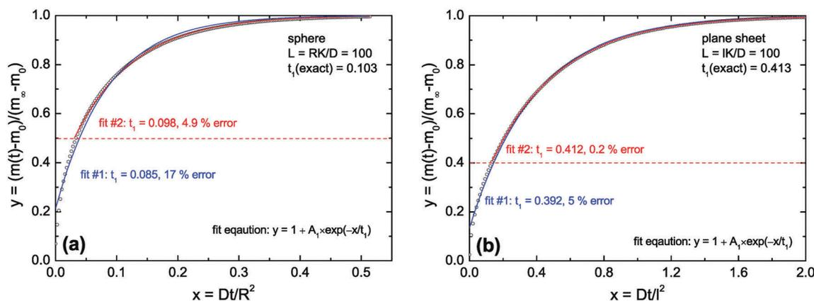
Fig. 2 Open points are calculated values for  $L = 100$  (diffusion controlled regime). In (a) eqn (3) was used and in (b) eqn (8) was used (the first six roots in both cases). Fit #1: The complete set of calculated data was fitted by eqn (13). Fit #2: All calculated data in the range  $0 \leq y \leq y_{\text{start}}$  were excluded from the fitting procedure, with  $y_{\text{start}} = 0.5$  in the case of a sphere (a) and  $y_{\text{start}} = 0.4$  in the case of a plane sheet (b).
