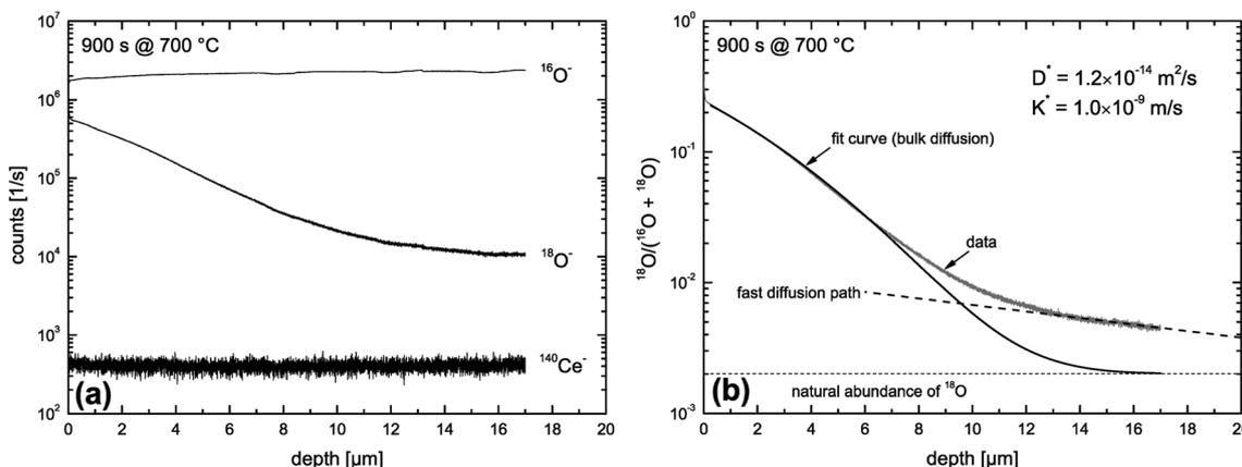
**Fig. 9** SIMS depth profiles measured in a nominally undoped polycrystalline CeO<sub>2</sub> sample which was annealed for 900 s in 200 mbar <sup>18</sup>O<sub>2</sub> gas at 700 °C. (a) SIMS raw data. (b) Atomic fraction of <sup>18</sup>O computed by eqn (19).
