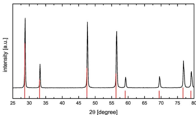
Fig. 4 XRD pattern of the synthesized CeO<sub>2</sub> sample (reference data according to ICDD PDF-00-034-0394<sup>23</sup> as red solid vertical lines).
