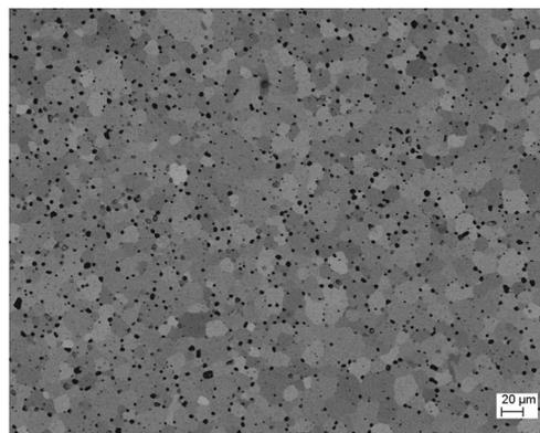
Fig. 5 SEM image of the sintered CeO<sub>2</sub> pellet with a grain size of about 20 μm and a density of 93% (Angle Selective Backscatter detector).
