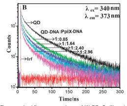
**Fig. 7** Time-resolved fluorescence decay of (A) QD-Pp IX conjugate and (B) QD-DNA-Pp IX assembly recorded for solutions with varying ratios of donor and acceptor. Irf: instrument response function.
