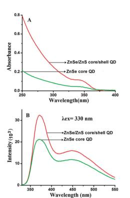
Fig. 1 (A) UV-visible absorption and (B) fluorescence spectra of ZnSe core and ZnSe-ZnS core—shell QDs.
