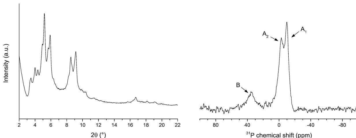
Fig. 2 Powder XRD pattern (left) and <sup>31</sup>P MAS NMR spectra (right) of LSK-15. NMR signals are labelled according to phosphorus oxidation state: A<sub>1</sub> ( $-10$  ppm) and A<sub>2</sub> ( $-6$  ppm) for phosphine and B ( $35$  ppm) for phosphine oxide. Adapted from ref. 12. Copyright 2014 American Chemical Society.
