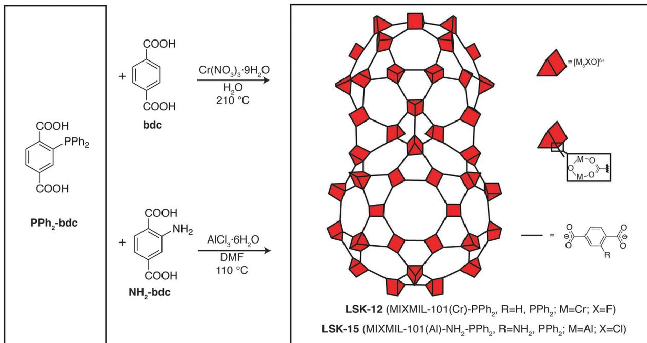
Fig. 1 Synthesis and schematic representation of P-MOFs with MIL-101 topology.
