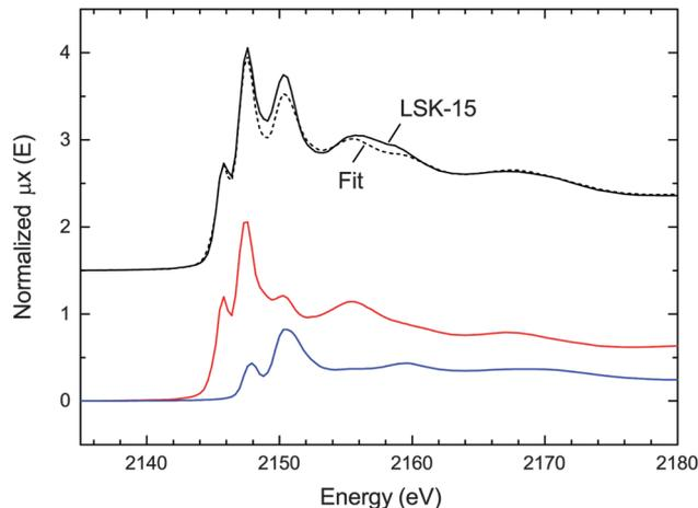
**Fig. 5** P K-edge XANES spectrum of LSK-15 (black) with the linear fit (dashed line) and the two weighted contributions of PPh<sub>2</sub>-bdc (red) and POPh<sub>2</sub>-bdc (blue).
