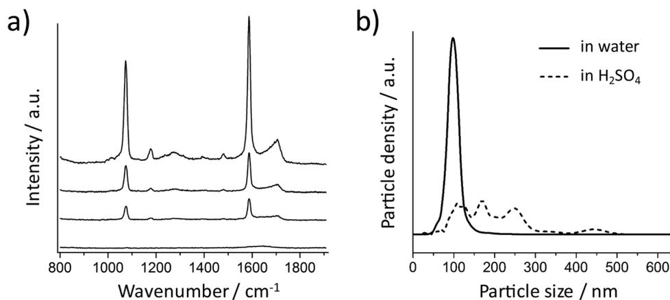
Fig. 3 (a) SERS spectra of 4-MBA on Au NPs (without silica shell) recorded at different times after suspension in 10 mM  $\text{H}_2\text{SO}_4$  solution. From bottom to top: 0 (before addition of acid), 1, 10, and 30 minutes. (b) Particle size distribution of the Au NPs with 4-MBA SAM in water (solid line) and after 30 minutes in the 10 mM  $\text{H}_2\text{SO}_4$  solution (dashed line).
