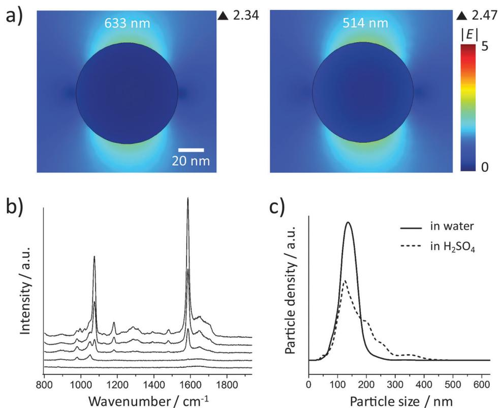
**Fig. 5** (a) FEM simulation of the incident electric field amplitude  $|E|$  distribution on a 80 nm Ag sphere upon 633 (left) and 514 (right) nm excitation. (b) SERS spectra of 4-MBA on the 80 nm Ag NPs measured at different time periods after the addition of 1 M  $\text{H}_2\text{SO}_4$ . From bottom to top: 0, 1, 30, 60, and 100 minutes. (c) Size distribution of the Ag NPs with 4-MBA SAM in water and after 100 minutes incubation in  $\text{H}_2\text{SO}_4$ .
