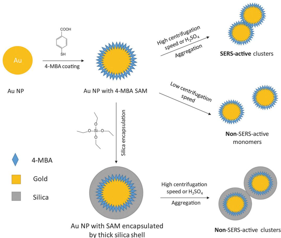
**Fig. 1** Preparation of SERS-active NP clusters and non-SERS-active Au NP monomers, both coated with a SAM of Raman reporter molecules (4-MBA). When the NPs are washed at a high centrifugation speed or are resuspended in acidic (or salt) solution, SERS-active clusters are formed (top right). Low speed centrifugation (middle right) and encapsulation within a thick silica shell (bottom right) leads to non-SERS-active colloids without plasmonic coupling between NPs.
