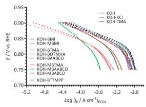
Fig. 7 The Tafel plots at 25 °C of the Pt/C-coated GC disk electrode in the  $O_2$ -saturated aqueous KOH (1 mol dm $^{-3}$ ) electrolytes with and without addition of 1 mmol dm $^{-3}$  of each of the additives (derived from the data in Fig. ESI3 and ESI4†). The kinetic current densities were normalised to the ECSAs presented in Fig. 1.
