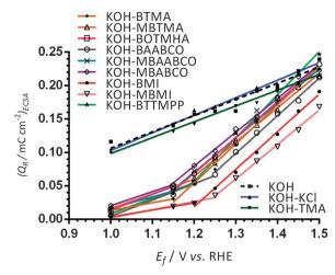
Fig. 4 The charge densities  $Q_R$  at 25 °C obtained by integration of the reduction peaks (potential range +0.9 to +0.45 V vs. RHE) in the reverse scans of CVs presented in Fig. 3 (with increasing upper anodic potential limits  $[E_f]$ ). The Pt/C-coated GC disk electrodes were submerged in N<sub>2</sub>-saturated aqueous KOH (1 mol dm<sup>-3</sup>) electrolytes with and without the addition of 1 mmol dm<sup>-3</sup> of organic cationic species (and KCl).
