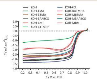
**Fig. 6** The LSVs at 25 °C for the Pt/C-coated GC-RDEs in  $O_2$ -saturated aqueous KOH (1 mol dm $^{-3}$ ) electrolytes with and without addition of 1 mmol dm $^{-3}$  of each of the cationic molecules studied. Scan rate = 5 mV s $^{-1}$  and RDE rotation rate = 1600 rpm. The currents presented here were normalised to the RDE geometric surface area.
