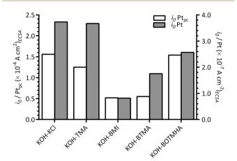
**Fig. 10** A comparison of apparent exchange current densities  $(i_0)$  at 25 °C with the KCl-, TMA-, BTMA-, BOTMHA-, and BMI-(1 mmol dm<sup>-3</sup>)-containing aqueous KOH (1 mol dm<sup>-3</sup>) electrolytes using data from this study (Pt/C-coated GC-disk electrode – filled bars [y2-axis]) and data recorded in the previous study (Pt<sub>pc</sub>-disk electrode – unfilled bars [y1-axis]).
