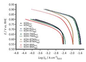
Fig. 12 A comparison of Tafel plots with the KCl-, TMA-, BTMA-, and BMI-(1 mmol dm $^{-3}$ )-containing aqueous KOH (1 mol dm $^{-3}$ ) electrolytes measured using a Pt/C (symbols) and a Ag/C (lines) coated GC-disk electrodes.
