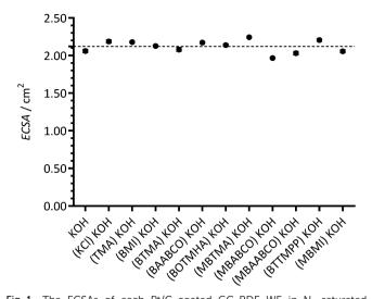
Fig. 1 The ECSAs of each Pt/C-coated GC-RDE WE in N2-saturated aqueous KOH (1 mol dm<sup>-3</sup>) electrolytes at 25 °C before addition of  $1~\mathrm{mmol~dm^{-3}}$  of the bracketed model cationic molecules (or KCl). Scan rate =  $50 \text{ mV s}^{-1}$ . Error bars are the confidence intervals at the 95%confidence level (n = 3 repeated CVs on each GC-RDE WE). The dashed line gives the mean value of all ECSAs collected with all WEs
