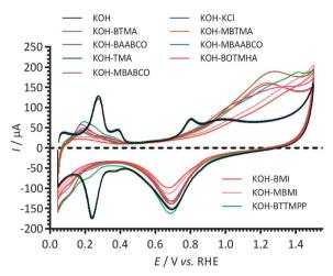
Fig. 2 Cyclic voltammograms of a Pt/C-coated GC disk electrode in  $N_2$ -saturated aqueous KOH (1 mol dm<sup>-3</sup>) electrolytes at 25 °C with and without addition of 1 mmol dm<sup>-3</sup> of cationic molecules and KCl (control experiment for  $Cl^-$  spectator anions). Scan rate = 50 mV s<sup>-1</sup>.
