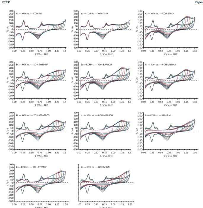
Fig. 3 Cyclic voltammograms of Pt/C-coated GC disk electrodes in N<sub>2</sub>-saturated aqueous KOH (1 mol dm<sup>-3</sup>) electrolyte at 25 °C without (--- dashed lines) and with addition (— solid lines) of 1 mmol dm<sup>-3</sup> of: (A) KCl, (B) TMA, (C) BTMA, (D) BOTMHA, (E) BAABCO, (F) MBTMA, (G) MBAABCO, (H) MBABCO, (I) BMI, (J) BTTMPP and (K) MBMI. The CVs were recorded with progressively higher upper potential limits ( $E_t$ ) up to 1.5 V vs. RHE. Scan rate = 50 mV s<sup>-1</sup>.
