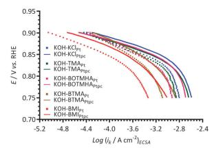
**Fig. 9** A comparison of Tafel plots with the KCl-, TMA-, BTMA-, BOTMHA-, and BMI-(1 mmol dm $^{-3}$ )-containing aqueous KOH (1 mol dm $^{-3}$ ) electrolytes using data from this study (Pt/C-coated GC-disk electrode – squares) and data recorded in the previous study (Pt<sub>pc</sub>-disk electrode – solid lines).<sup>12</sup>
