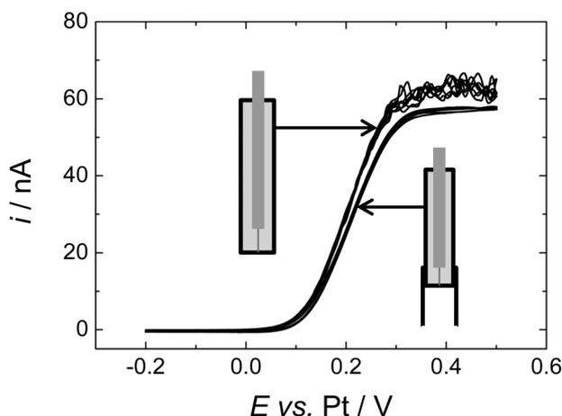
**Fig. 4** Cyclic voltammetry in 1.42 mM DMFc in supercritical CO<sub>2</sub> with 15 wt% MeCN containing 20 mM [NBu<sub>4</sub>][BF<sub>4</sub>] supporting electrolyte at 309 K. The working electrodes were both nominally 50  $\mu$ m diameter platinum discs with and without a baffle, the counter and reference electrode were 0.5 mm diameter platinum wires.  $p = 17.58$  MPa,  $p = 17.49$  MPa respectively. Sweep rate 10 mV s<sup>-1</sup> for all electrodes.
