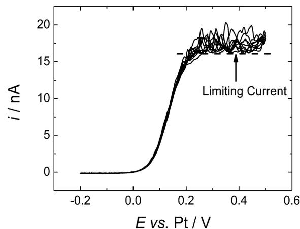
Fig. 3 Cyclic voltammograms in 0.43 mM DMFc in supercritical CO<sub>2</sub> with 15 wt% MeCN containing 20 mM [NBu<sub>4</sub>][BF<sub>4</sub>] supporting electrolyte.  $T = 309$  K.  $p = 17.60$  MPa. The working electrodes was a 50 μm diameter platinum disc, the counter and reference electrode were 0.5 mm diameter platinum wires. Sweep rate 10 mV s<sup>-1</sup>.
