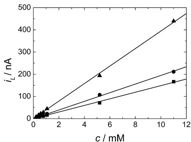
**Fig. 5** Plot of diffusion limited current versus the decamethylferrocene concentration for a series of cyclic voltammograms in supercritical CO<sub>2</sub> with 15 wt% MeCN and 20 mM [NBu<sub>4</sub>][BF<sub>4</sub>] electrolyte.  $T = 309$  K,  $p = 17.24$ – $17.72$  MPa. The working electrodes were a 20 (■), 25 (●) and 50  $\mu$ m (▲) diameter platinum disc, the counter and reference electrode were 0.5 mm diameter platinum wires.
