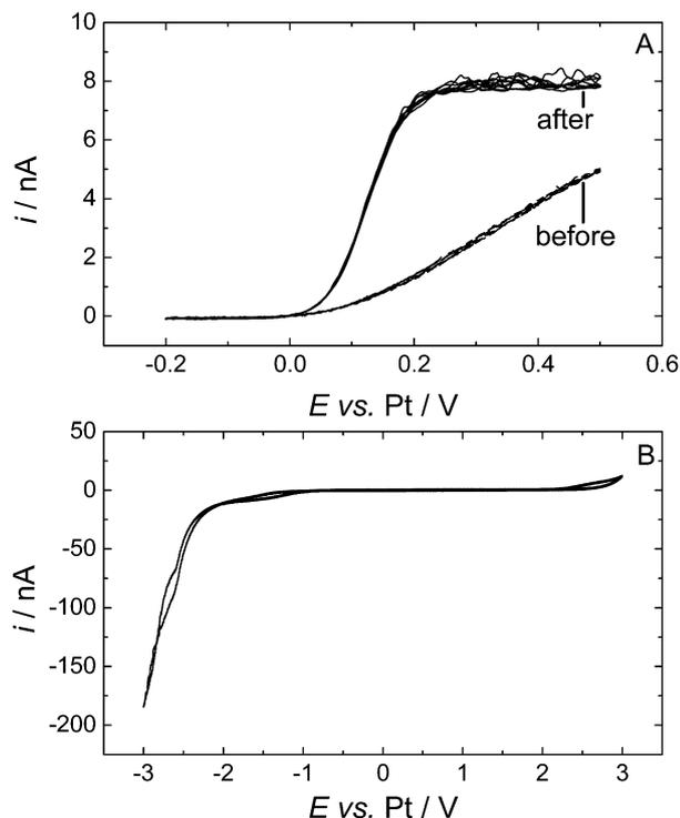
Fig. 1 Cyclic voltammety of 0.43 mM DMFc in supercritical CO<sub>2</sub> with 15 wt% MeCN containing 20 mM [NBu<sub>4</sub>][BF<sub>4</sub>] supporting electrolyte at 309 K. The working electrodes were a 25 μm diameter platinum disc, the counter and reference electrode were 0.5 mm diameter platinum wires.  $p_A \approx 17.50$  MPa,  $p_B = 17.43$  MPa. Voltammograms for (A) were recorded at 10 mV s<sup>-1</sup>, (B) at 100 mV s<sup>-1</sup>.
