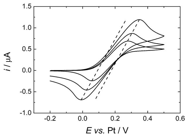
**Fig. 7** Cyclic voltammograms in 0.638 mM DMFc in supercritical  $\text{CO}_2$  with 15 wt% MeCN containing 20 mM  $[\text{NBu}^n_4][\text{BF}_4]$  supporting electrolyte.  $T = 309 \text{ K}$ .  $p = 17.51 \text{ MPa}$ . The working electrodes was a 0.5 mm diameter gold disc, the counter and reference electrode were 0.5 mm diameter platinum wires. Sweep rate 100, 200 and 500  $\text{mV s}^{-1}$ .
