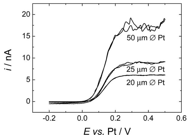
Fig. 2 Cyclic voltammetry of 0.43 mM DMFc in supercritical CO<sub>2</sub> with 15 wt% MeCN containing 20 mM [NBu<sub>4</sub>][BF<sub>4</sub>] supporting electrolyte at 309 K. The working electrodes were a 20, 25 and 50 μm diameter platinum disc, the counter and reference electrode were 0.5 mm diameter platinum wires.  $p = 17.51$  MPa,  $p = 17.55$  MPa,  $p = 17.60$  MPa respectively. Sweep rate 10 mV s<sup>-1</sup> for all electrodes.
