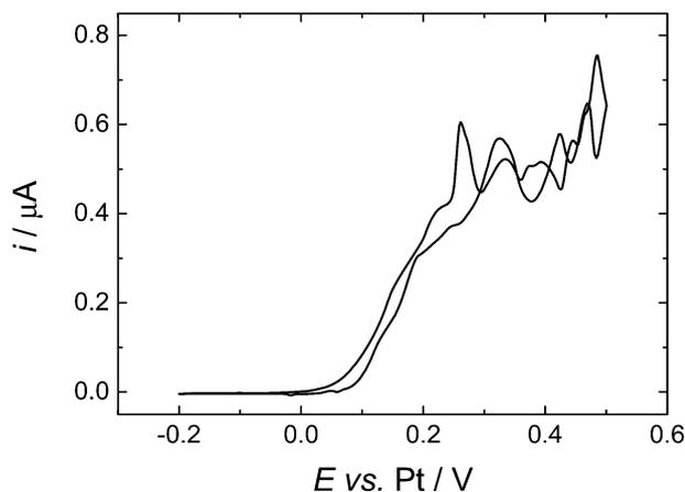
Fig. 8 Cyclic voltammetry in 0.638 mM DMFc in supercritical CO<sub>2</sub> with 15 wt% MeCN containing 20 mM [NBu<sub>4</sub>][BF<sub>4</sub>] supporting electrolyte.  $T = 309$  K,  $p = 17.51$  MPa. The working electrode was a 0.5 mm diameter gold disc, the counter and reference electrode were 0.5 mm diameter platinum wires. Sweep rate 10 mV s<sup>-1</sup>.
