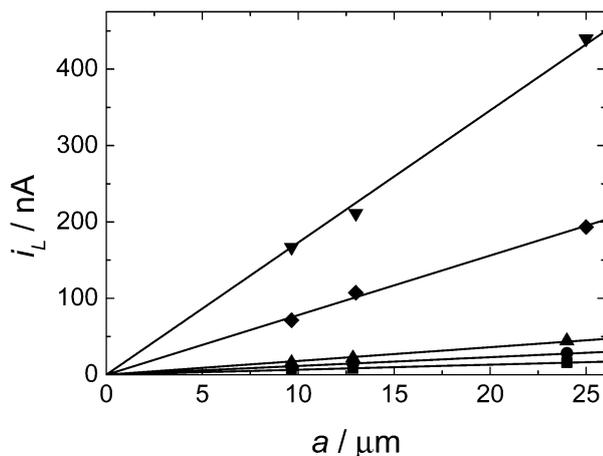
**Fig. 6** Plot of diffusion limited current versus the electrode radii for a series of cyclic voltammograms in supercritical  $\text{CO}_2$  with 15 wt% MeCN and 20 mM  $[\text{NBu}^n_4][\text{BF}_4]$  electrolyte.  $T = 309 \text{ K}$ .  $p = 17.24\text{--}17.72 \text{ MPa}$ . The concentrations were 0.43 (■), 0.78 (●), 1.07 (▲), 5.20 (◆), and 11.0 mM (▼). The counter and reference electrode were 0.5 mm diameter platinum wires.
