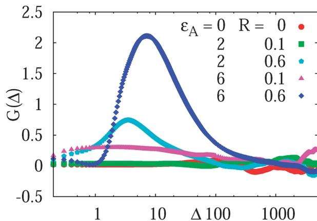
Fig. 9 Non-Gaussianity parameter (18) computed for the tracer diffusion on a lattice of sticky obstacles, the parameters are indicated. As a reference for almost perfect Gaussian behaviour  $G = 0$ , we present the non-Gaussianity parameter for vanishingly small, inert obstacles. The length of individual simulated trajectories is  $T = 10^4$ .
