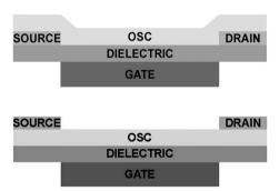
Fig. 1 Schematic view of an organic field-effect transistor (OFET). (top) Bottom-gate bottom-contact (BGBC) configuration. (bottom) Bottomgate top-contact (BGTC) configuration.
