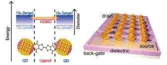
Fig. 11 Left: energy level diagram of a coupled organic-inorganic nanostructure interface. In this example, the inorganic 1Sh state is tuned by the QD diameter to align with the HOMO of the OSC as for instance in ref. 127. However, the same concept may be imagined for the 1Se of the QD and the LUMO of the OSC. Right: an idealized schematic of a field effect transistor of this COIN
