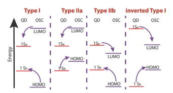
Fig. 1 Simplified schematic of different types of energy alignment between the lowest electron (1Se) as well as the highest hole level (1Sh) of a quantum dot (QD) and the highest occupied molecular orbital (HOMO) as well as lowest unoccupied molecular orbital (LUMO) of an organic semiconductor (OSC) ligand.
