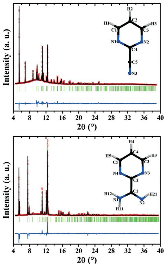
Fig. 3 Rietveld refinement plots ( $\lambda = 0.68884 \text{ \AA}$ ) of 2-cyanopyrimidine (top) and pyrimidine-2-carboximidamide (bottom). Experimental and calculated data are shown in red symbols and black line, respectively. Blue line shows the difference curve, while green marks show Bragg positions. Insets show molecular structures of 2-cyanopyrimidine and pyrimidine-2-carboximidamide.
