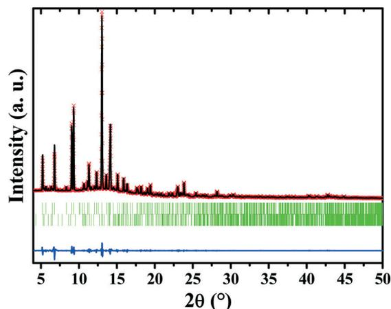
Fig. 8 Le Bail fit to the synchrotron radiation X-ray powder pattern ( $\lambda = 0.821693 \text{ \AA}$ ) of the sample obtained by the reaction of 2-cyanopyrimidine with pyrimidine-2-carboximidamide. Experimental and calculated data are shown in red symbols and black line, respectively. Blue line shows the difference curve, while green marks show Bragg positions for  $\alpha$ -TPymT (top row) and  $\beta$ -TPymT (bottom row).
