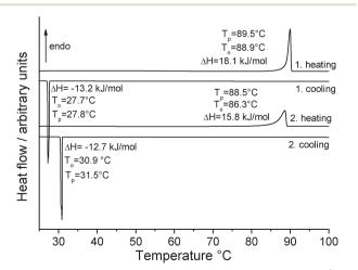
Fig. 9 DSC heating and cooling curves for form 1t at 1 °C min<sup>-1</sup>; the peak  $(T_p)$  and onset  $(T_o)$  temperatures are given in °C and the enthalpy  $\Lambda H$  in kJ mol<sup>-1</sup>.
