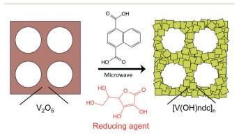
Fig. 1 Scheme of the replication of the V<sub>2</sub>O<sub>5</sub> sacrificial template into [V(OH)ndc]<sub>n</sub> polycrystalline macrostructures.
