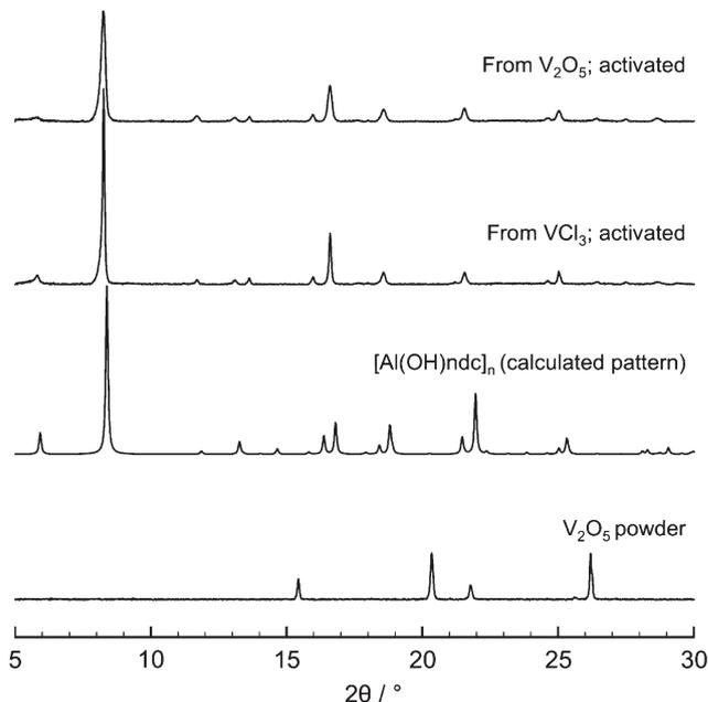
Fig. 2 XRD pattern of the activated [V(O)ndc]<sub>n</sub> obtained from V<sub>2</sub>O<sub>5</sub> and from VCl<sub>3</sub>, calculated pattern of [Al(OH)ndc]<sub>n</sub> and XRD pattern of the commercial V<sub>2</sub>O<sub>5</sub> powder.
