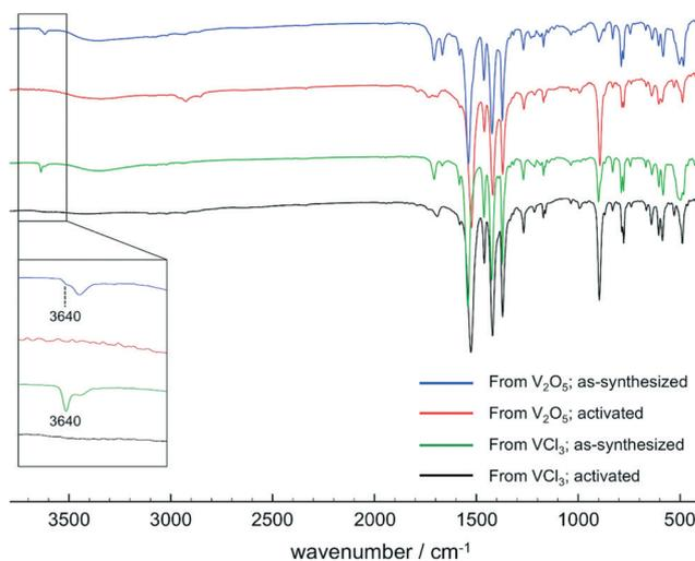
Fig. 3 IR spectra of [V(OH)ndc]<sub>n</sub> before and after activation obtained from V<sub>2</sub>O<sub>5</sub> and from VCl<sub>3</sub>. The inset highlights the spectral region ranging from 3010 cm<sup>-1</sup> to 3750 cm<sup>-1</sup>.
