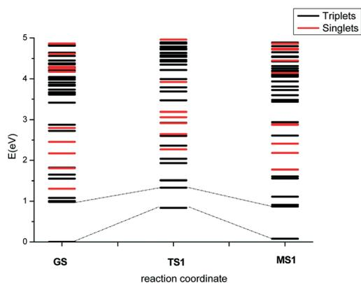
Fig. 7 Energy profiles for the GS  $\rightarrow$  MS1 transition in the ground and photoexcited states. Triplet and singlet states are indicated by black and red lines, respectively. The excited states were computed at the TD-DFT/M06/LANL2DZ/6-311++G(d,p) level of theory with water as a continuum.
