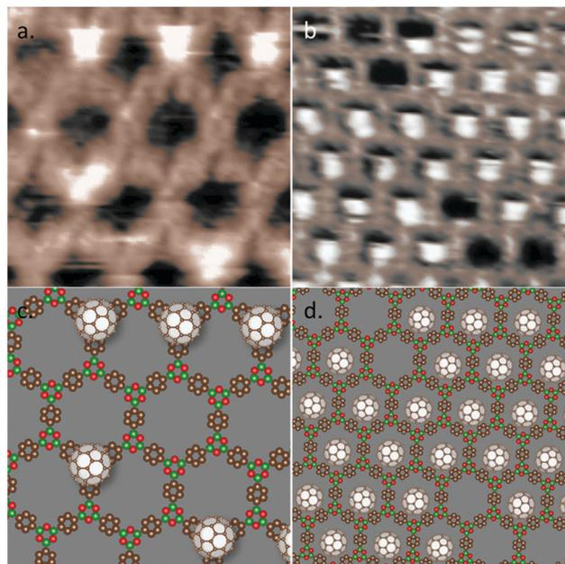
**Fig. 2** H/G structures at the solution/solid interface. The images in (a) and (b) show the observed fullerene adsorption geometries, denoted as top site and pore site, respectively. The structures in (c) and (d) show proposed models for these adsorption sites. Scanning conditions: bias voltage  $U_t = -800$  mV, tunneling current  $I = 100$  pA. Image widths (a) 5.3 nm and (b) 7.7 nm.
