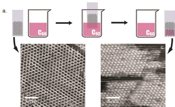
Fig. 3 Schematic illustration of dipstick preparation of COF-1/fullerene H/G structure. The image in (b) shows the as-synthesized COF-1 on HOPG. Following immersion into a solution of  $C_{60}$  in heptanoic acid (a) and subsequent drying, STM images like that in (c) reveal COF-1 populated with  $C_{60}$  guest molecules. Imaging parameters: voltage  $U_t = -800$  mV, tunneling current  $I = 100$  pA.
