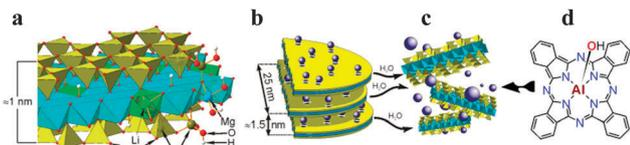
Fig. 1 Composition of LAPONITE<sup>®</sup> (a) and the dimensions of the disks (b), the solubility behavior (c) and adsorption of a dye (d), here demonstrated with Al(OH)Pc.
