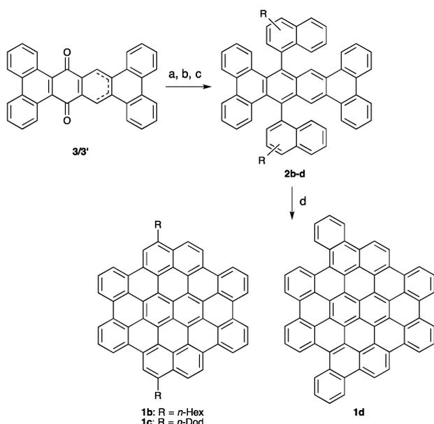
**Scheme 3** Synthesis of tetrabenzocircumpyrene derivatives. (a) ArBr,  $n$ -BuLi, Et<sub>2</sub>O/toluene, rt, 2 h (**2b**, 32%; **2c**, 26%; **2d**, 38%); (b) HI, AcOH,  $100$  °C, 16 h; (c) DDQ, toluene,  $70$  °C, 1 h; and (d) FeCl<sub>3</sub>, CH<sub>3</sub>NO<sub>2</sub>/CH<sub>2</sub>Cl<sub>2</sub>, rt, 16 h (**1b**, 85%; **1c**, 54%; **1d**, 64%).
