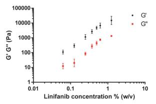
Fig. 4 Storage modulus (G') (black circle) and loss modulus (G'') (red square) *versus* linifanib concentration (% (w/v)) in 0.5% (v/v) DMSO-water. All measurements were carried out in triplicate and the mean calculated. Error bars represent standard deviation.
