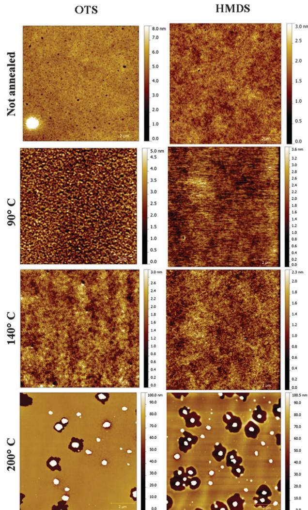
Fig. 2 Topographical atomic force microscopy images ( $10 \mu\text{m} \times 10 \mu\text{m}$ ) of spin-coated ICBA films ( $10 \text{ mg mL}^{-1}$  in chloroform) annealed at different temperature on either OTS or HMDS (annealing time: 1 h). For consistency with the device architecture, the imaged films are realized on a SiO<sub>2</sub> substrate.
