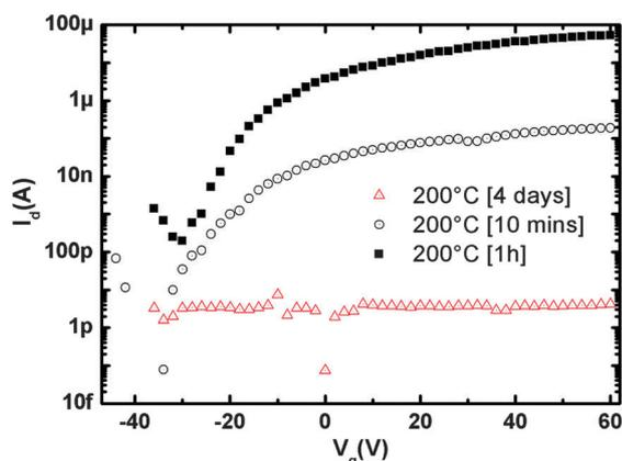
Fig. 4 Comparative transfer curves ( $I_d$ – $V_g$ ) of typical ICBA-based thin-film transistors with OTS-treated SiO<sub>2</sub> where the active layer underwent annealing at 200 °C for 4 days, 1 h or 10 minutes, respectively. ( $W = 10$  mm,  $L = 20$  μm;  $V_d = +60$  V).
