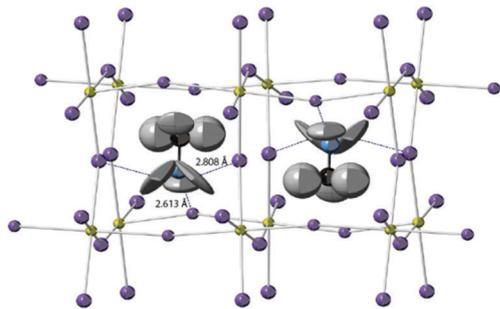
**Fig. 1** The unit cell of MAPbI<sub>3</sub> at 100 K viewed close to *a*-axis the showing ADPs as 90% probability ellipsoids; lead yellow, iodine purple, carbon black, nitrogen blue and hydrogen grey.
