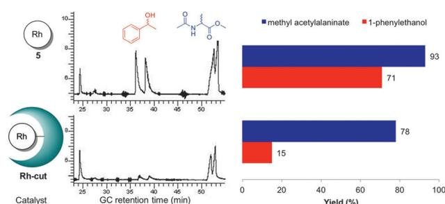
**Fig. 2** Reaction outcome of the competitive hydrogenation of acetophenone vs. methyl 2-acetamidoacrylate (right) and the corresponding chiral GC chromatograms (center) comparing catalysts **5** [Rh(cod)(SI)Mes)Cl] and **Rh-cut** (left).
