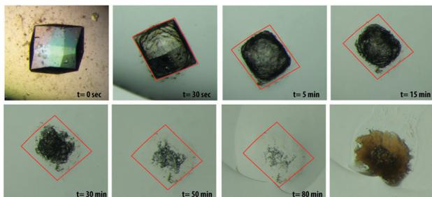
Fig. 3 Dissolution sequence of a lysozyme crystal grown in hydrogel 1. Crystal extracted from the gel was placed in a water drop and allowed to dissolve ( $t = 0$  s). A red square is drawn around the remaining hydrogel. The last picture was taken after partially drying the remaining gel framework.
