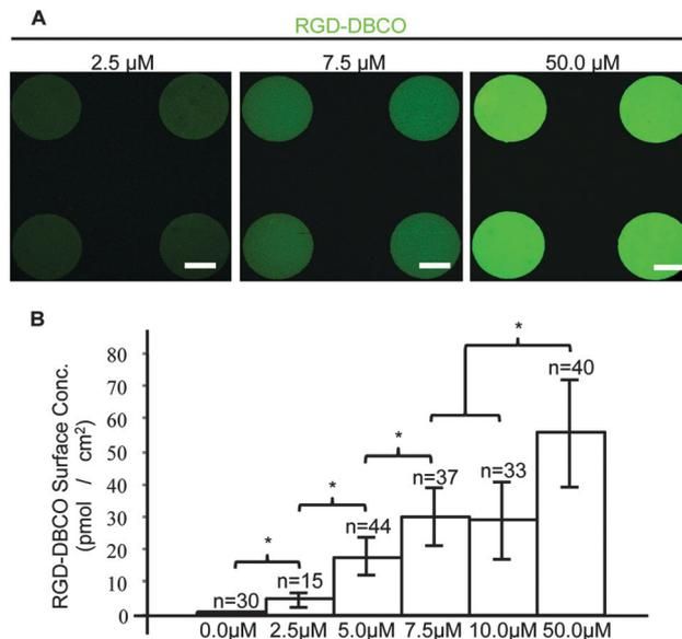
Fig. 1 (A) Fluorescent images of micropatterned PEGMA brushes conjugated with RGD-DBCO at varying reaction concentrations, 150  $\mu$ m scale bars. (B) Surface density of RGD-DBCO on micropatterned substrates across all reaction concentrations, \* $p < 0.05$ .
