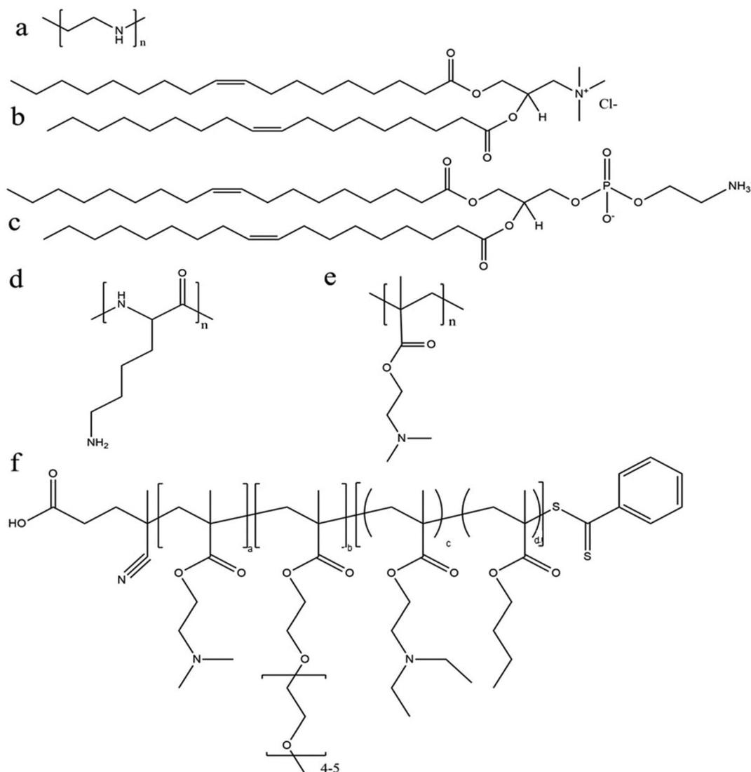
**Fig. 4** Chemical structure of some representative polymers and lipids used for mRNA delivery: (a) polyethylenimine (PEI); (b) 1,2-dioleoyl-3-trimethylammonium-propane (chloride salt) (DOTAP); (c) 1,2-dioleoyl-*sn*-glycero-3-phosphoethanolamine (DOPE); (d) poly(L-lysine) (PLL); (e) poly(2-(dimethylamino)ethyl methacrylate) (p(DMAEMA)); and (f) poly(DMAEMA-PEGMA-DEAEMA-co-BMA).
