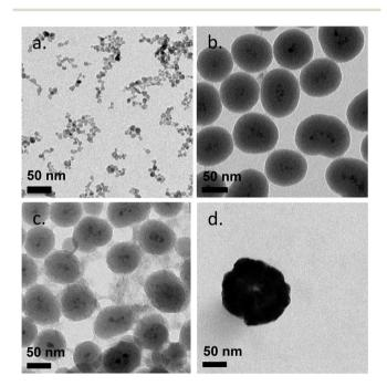
Fig. 2 Transmission electron microscopy (TEM) images of naked SPION (a), SiO<sub>2</sub>-SPION (b), TiO<sub>2</sub>-SPION (c) and gold-SPION (d).
