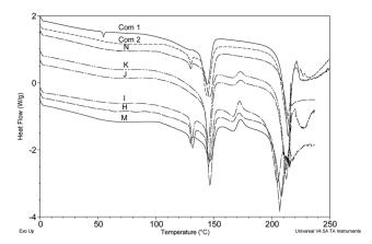
Fig. 7 DSC thermograms of seven selected cases all containing lactose as the bulk excipient and including Com 1 and Com 2 for comparison. Note the apparent absence of amorphous lactose content in both licit samples and Case N.
