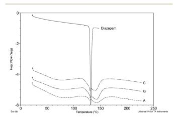
Fig. 8 DSC thermograms of Cases A, C and G containing diazepam and an (as yet) unidentified excipient.
