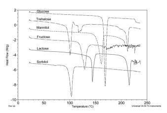
Fig. 4 DSC thermograms of six sugars commonly used as tablet excipients.
