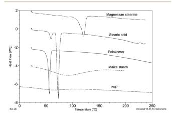
Fig. 6 DSC thermograms of five common tablet excipients for illustrative purposes.
