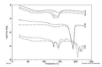
Fig. 10 DSC thermograms of a selection of cases grouped by bulk excipient. Note the significant differences between Cases D and F which both contain lactose.
