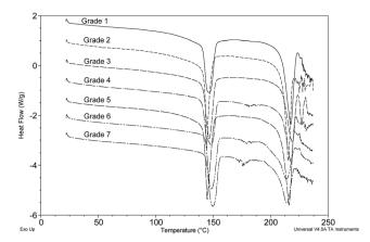
Fig. 5 Grade 1-Lactose B.P. (supplier unknown); Grade 2-Granulac™230; Grade 3-Lactopress™150; Grade 4-Lactopress™5D; Grade 5-Pharmatose™80; Grade 6-Lactopress™175; Grade 7-Lactopress™300.
