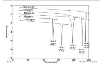
Fig. 3 DSC thermograms of five different benzodiazepines at a heating rate of 10  $^{\circ}$ C min $^{-1}$  indicating the individual melting points. Values of  $T_{\rm onset}$  and  $T_{\rm max}$  and the enthalpy of fusion (J g $^{-1}$ ) are indicated for each pure compound.
