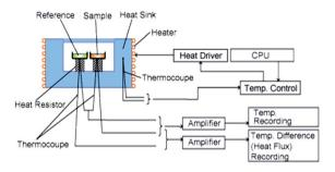
Fig. 1 Schematic diagram of a heat flux differential scanning calorimeter (DSC). Courtesy of http://Hitachi-Hightec.com.
