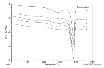
Fig. 9 DSC thermograms of Cases B, E, L and P containing Emcompress™ as the bulk excipient.
