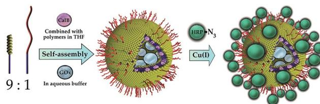
Fig. 4 Site-specific immobilization of an enzyme cascade in polymersome nanocontainers: *Candida antarctica* Lipase B (CalB) is embedded in the polymersome membrane, glucose oxidase (GOx) is entrapped in the inner lumen of the container and horseradish peroxidase (HRP) is attached to the outer polymersome surface by a Click chemistry approach. Reprinted from ref. 17 with permission of John Wiley and Sons.
