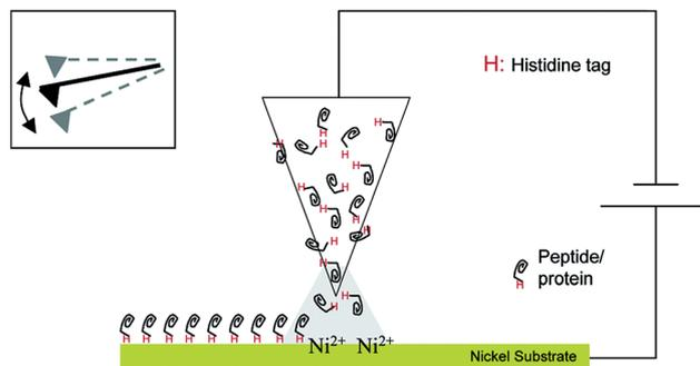
Fig. 1 Site-specific immobilization of polyhistidine-tagged proteins to a Ni-substrate by dip-pen-nanolithography. Reprinted (adapted) with permission from.<sup>39</sup> Copyright (2015) American Chemical Society.
