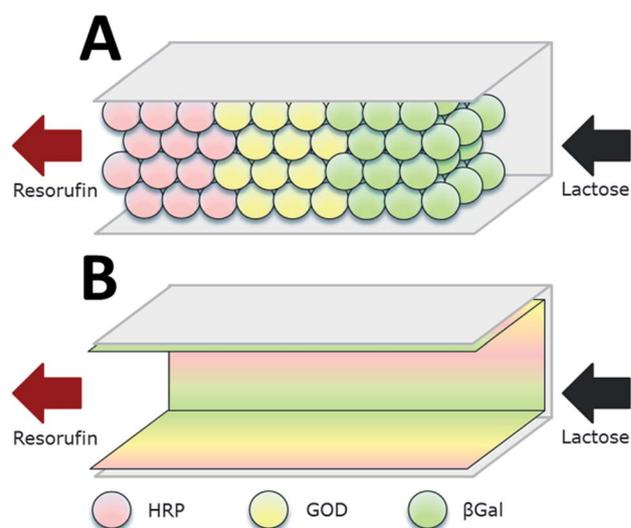
Fig. 5 Co-immobilization of  $\beta$ -galactosidase ( $\beta$ Gal, green), glucose oxidase (GOx, here GOD, yellow) and horseradish peroxidase (HRP, red) in a microfluidic channel by two approaches: (A) immobilization to microbeads that are subsequently packed in the channel. (B) direct attachment to the inner surface of the microchannels. The packed bed reactor (A) proved to be the more efficient approach. Reprinted from ref. 18 with permission of The Royal Society of Chemistry.
