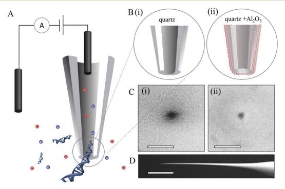
Fig. 1 A. Schematic of the experimental set up with nanopipette. B. Zoomed in schematic of the tip end of the (i) unmodified pipette (ii) Al<sub>2</sub>O<sub>3</sub>ALDmodified pipette. C. SEM characterization of the pore diameter (i) 25 nm and (ii) 7.5 nm. The scale bars are 40 nm. D. SEM image of the nanopipette tip (scale bar is 200 μm).
