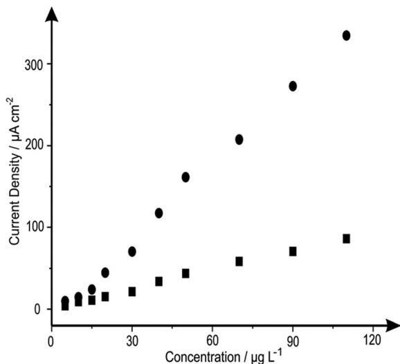
**Fig. 3** Analysis of the data presented in Fig. 2 in terms of plots of current density (of the peak heights) against increasing concentrations of lead(II) ions utilising the bSPEs (squares) and b<sup>2</sup>SPEs (circles). Deposition potential and time:  $-1.2$  V and 30 seconds respectively.
