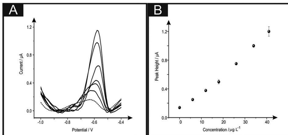
**Fig. 5** Square wave voltammograms obtained using different b<sup>2</sup>SPEs (A) in a drinking water sample in the absence (dashed line) and the result of increasing additions of lead(II) ions (solid lines). Standard addition plot (B) for the lead(II) ions within drinking water with corresponding errors bars. ( $N = 3$ ) A new electrode is used for each addition. Deposition potential and time of  $-1.2$  V and 30 seconds respectively.
