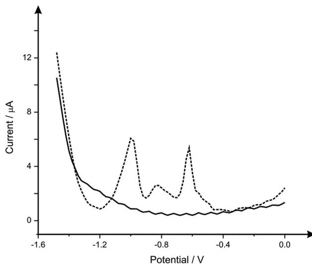
**Fig. 4** Square wave voltammograms obtained using the b<sup>2</sup>SPE within  $0.02$  M (pH 1.7) HCl (solid line) and the simultaneous detection of lead(II), cadmium(II) and zinc(II) at concentrations of  $8$ ,  $16$  and  $36 \mu\text{g L}^{-1}$  respectively (dashed line). Deposition potential and time of  $-1.5$  V and 120 seconds respectively.
