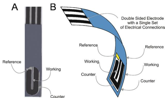
**Fig. 1** Optical image of a single side of a back-to-back screen-printed graphite microband (A) and a schematic depiction of the back-to-back configuration demonstrating the electrode lay-out and single point of electrical connection (B).
