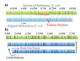
Fig. 4 (a) An example of a knot/backfold in an aligned molecule, blue, to the *E. coli* reference, green. The labels are shifted roughly 13 500 base pairs after the intensity spike (position in molecule shown in red). (b) An example of a folded region, highlighted by the purple arrow, within a molecule. The red insertion events do not align to the reference until the molecule is "unfolded".
