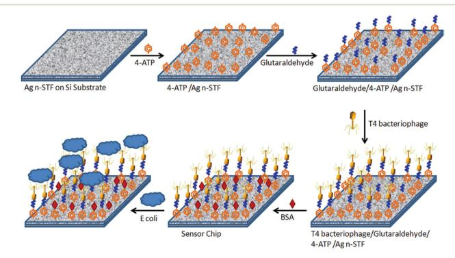
Fig. 1 Schematic of step by step sensor chip development.
