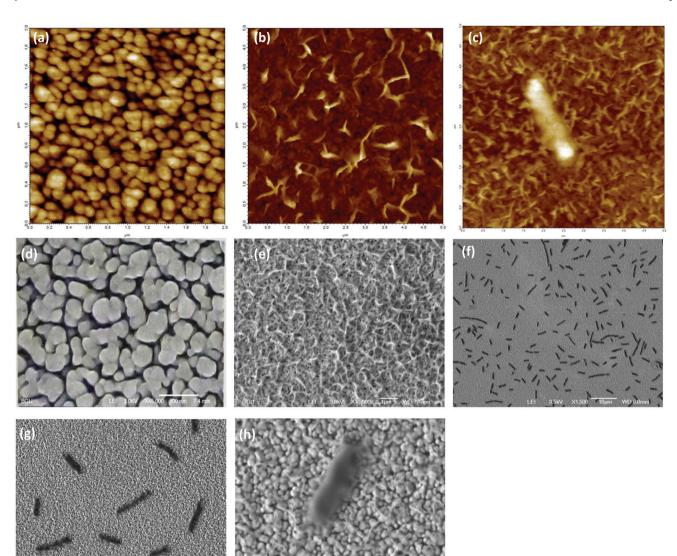
Fig. 2 AFM and SEM images of the nSTF sensor: (a), (d) before and (b), (e) after functionalization, respectively; (f), (g) SEM images of *E. coli B* attached to the sensor surface, and (c), (h) High resolution AFM and SEM images (respectively) of a single *E. coli B* attached to the sensor surface.
