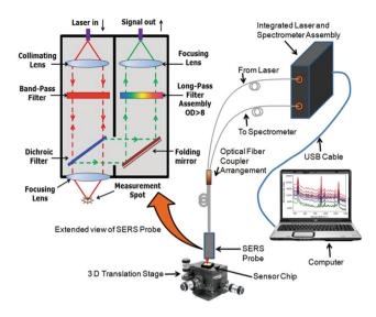
Fig. 3 Schematic of the experimental setup.
