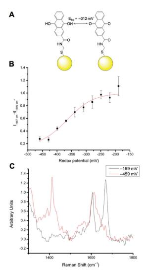
Fig. 2 AQ-NP nanosensor. (A): Equilibrium between oxidised and reduced AQ attached to a gold NP (yellow sphere, not to scale). (B): Calibration curve for AQ-NP nanosensors ( $R^2 = 0.96855$ ). (C): Representative spectra of fully oxidised (-189 mV) and fully reduced (-459 mV) AQ-NPs.
