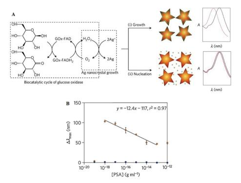
Fig. 11 (A) Schematic illustration of the proposed signal-generation mechanism by means of enzyme-guided crystal growth for the plasmonic ELISA assay. (B) Immunoassay for the ultrasensitive detection of PSA with GOx-labelled antibodies and of PSA (red) and BSA (green) spiked into whole serum. Reprinted with permission from ref. 87, copyright@2012, Nature Publishing group.
