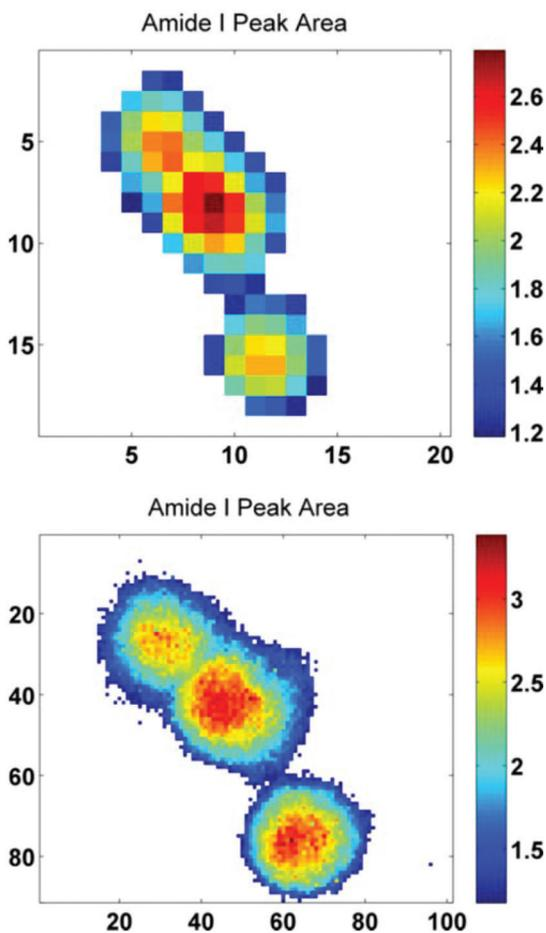
**Fig. 4** (top–bottom) Photo-micrograph taken with a 40 $\times$  objective, at a pixel resolution of 0.27  $\mu\text{m}$ . The amide I integrated peak area maps are presented for the raw spectral images acquired with normal and high magnification imaging modes respectively. The axes reflect the number of pixels, covering an area equivalent to  $\sim 100 \times 111 \mu\text{m}$ .
