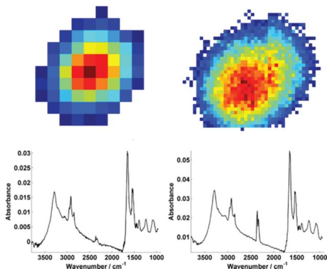
**Fig. 3** An individual isolated single cell from the raw data chemimaps for both low (left) and high (right) magnification modes. For both modes, the respective mean spectra calculated from individual pixel spectra (63 spectra for low mag. and 905 spectra for high mag.) are shown below the respective map.
