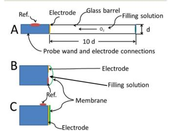
Fig. 4 Optimized electrode designs. (A) Whalen type showing recessed electrode; (B) Clark type, with both reference and indicating electrode behind the membrane, (C) membrane coated electrode, no filling solution.
