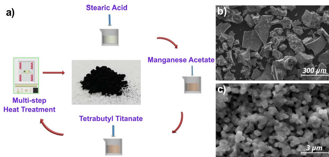
Fig. 1 (a) Schematic synthesis route for the synthesis of MnTiO 3 powders, (b) low magnification, and (c) high magnification FESEM images for the MnTiO 3 powders.
