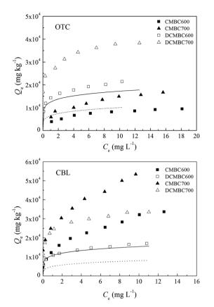
**Fig. 2** Comparison of the adsorption isotherms of oxytetracycline (OTC) and carbaryl (CBL) on original (CMBCs) and demineralized (DCMBCs) biochars. The solid and dotted lines represent the estimated Freundlich adsorption isotherms for CMBC700 and CMBC600, respectively.
