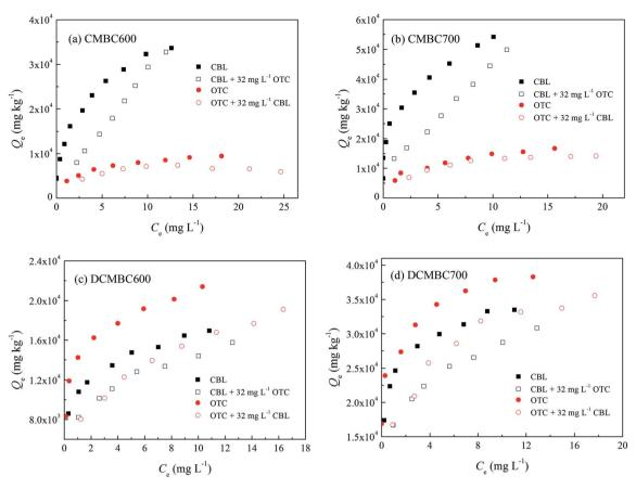
Fig. 4 Adsorption isotherms of carbaryl (CBL) and oxytetracycline (OTC) on original (CMBCs) and demineralized (DCMBCs) biochars with and without a co-solute ([OTC] or [CBL] =  $32 \text{ mg L}^{-1}$ ).
