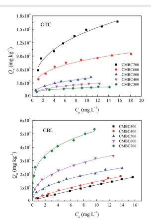
Fig. 1 Adsorption isotherms of oxytetracycline (OTC) and carbaryl (CBL) on original biochars pyrolyzed at different temperatures (300–700  $^{\circ}$ C).
